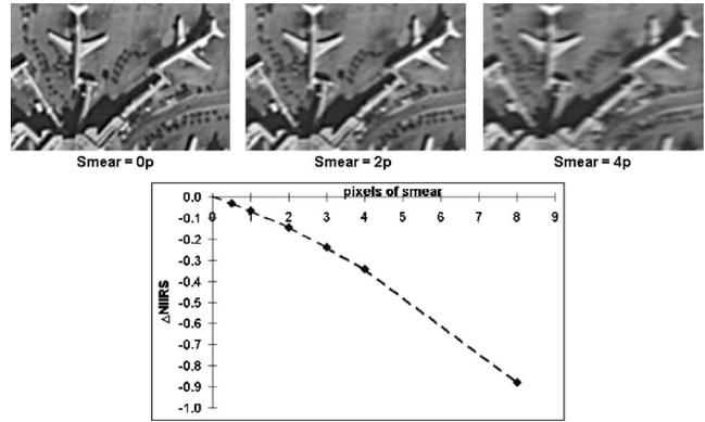
Figure 14. Image quality as a function of linear smear.
