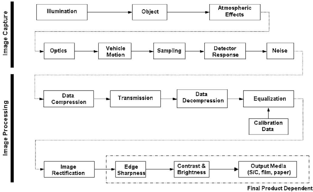
Figure 8. Image simulation process for an Earth-looking space imaging system models the image formation process.
