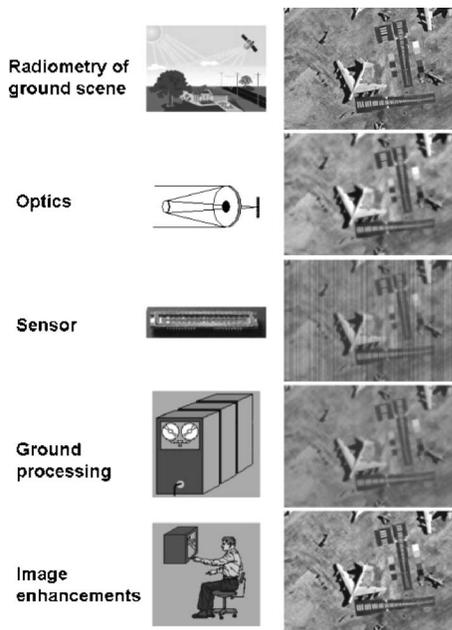
Figure 9. Series of images illustrating the effects of the imaging chain for an Earth-looking space imaging system design.
