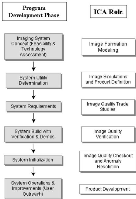
Figure 7. Image chain analysis plays a role through all phases of program development.
