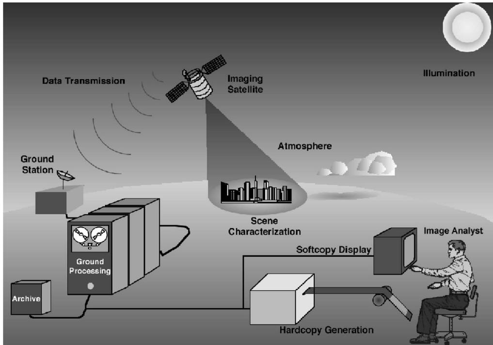
Figure 6. Imaging chain for an Earth-looking space imaging system.
