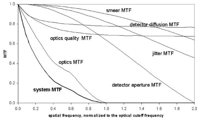
Figure 10. Individual MTF curves for a notional design and the final system MTF after the individual MTF curves have been multiplied together.
