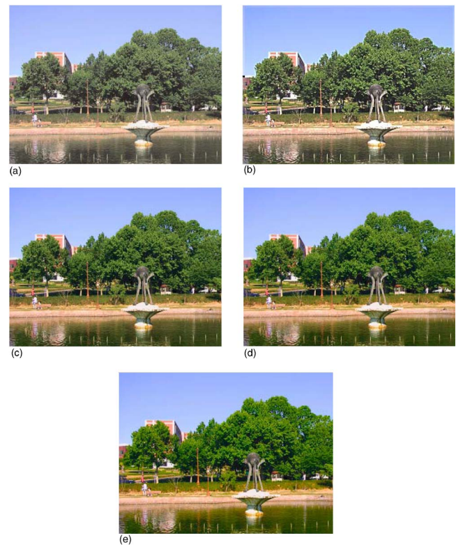
Figure 10. Enhanced park images under 10 000 lux: (a) lightness enhancement using the logarithmic function, (b) Monobe's method preserving the local contrast, (c) the proposed method with \beta=2.0 , (d) the proposed method with \beta=1.5 , and (e) the proposed method with \beta=1.0 .
