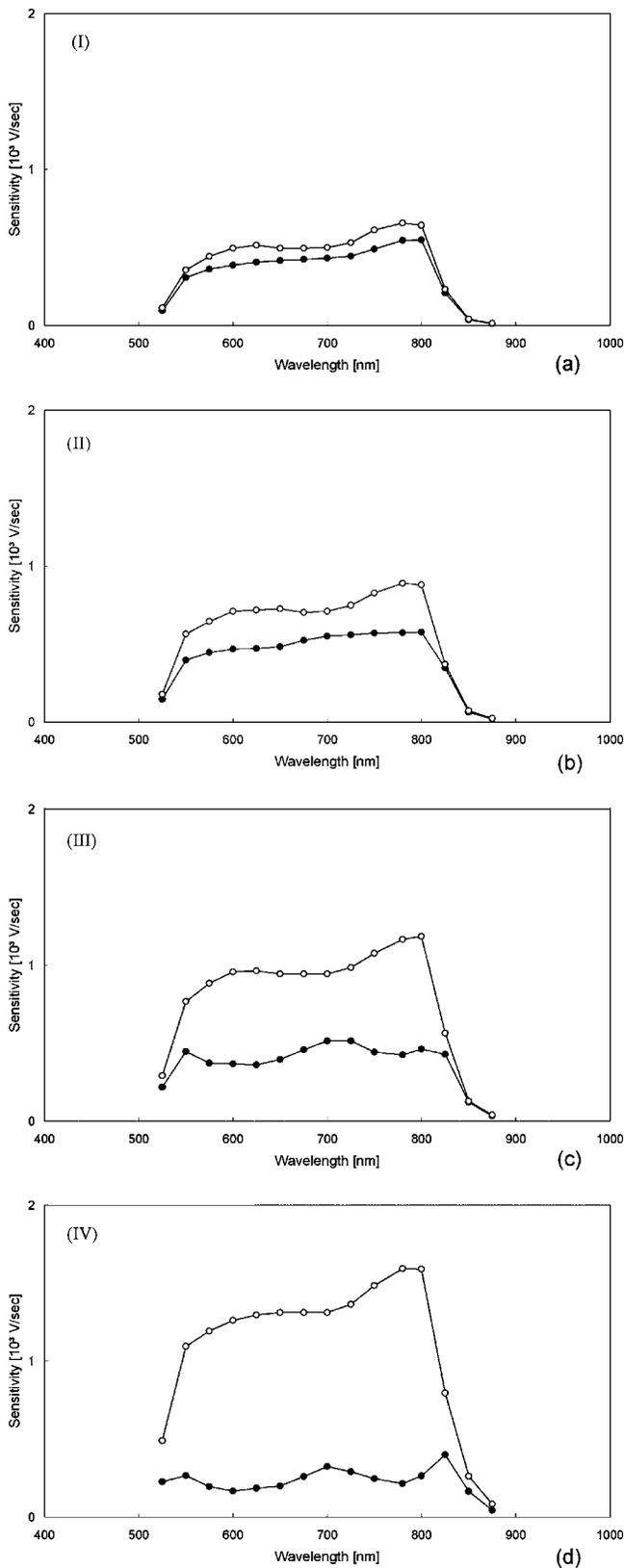
Figure 4. (a)–(d) Spectral sensitivities of both polarities: Open circles show the positive charging sensitivities and solid circles show the negative charging sensitivities; CGM concentration increases from (a) through (d).
