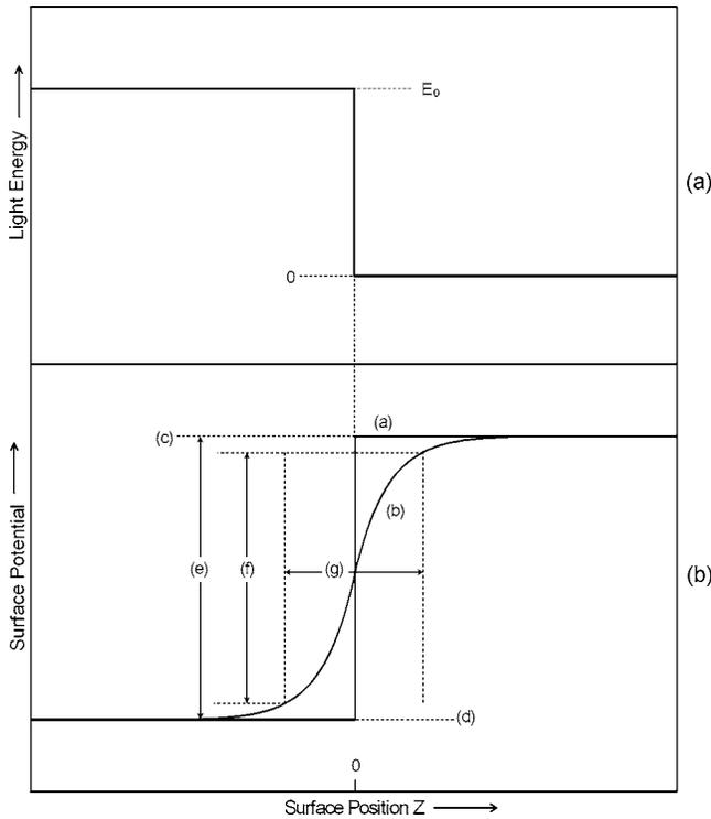
Figure 1. (a) Schematic illustration of light energy distribution at OPC surface, (b) illustration of edge degradation of latent image: (a) ideal potential profile, (b) degraded potential profile according to Eqs. (5) and (6), (c) dark potential, (d) light potential, (e) contrast potential, (f) practical contrast potential, and (g) edge width.
