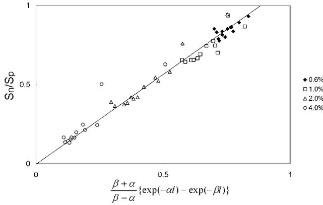
Figure 6. Correlation plot of  $(S_n/S_p)$  vs  $[(\beta+\alpha)/(\beta-\alpha)]\{\exp(-\alpha l) - \exp(-\beta l)\}$ . Dots are the calculated values from the data of spectral sensitivities of both polarities. Line is the least-squares approximation.
