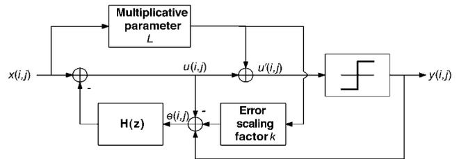
**Figure 9.** Block diagram of the proposed text-enhanced error diffusion.
