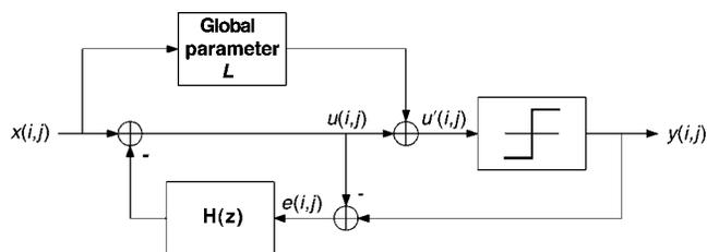
Figure 3. Conventional edge-enhanced error diffusion.
