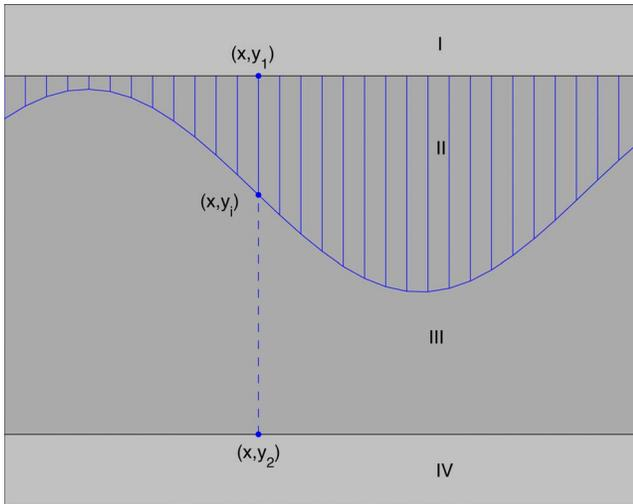
**Figure 1.** A schematic diagram of ink penetration consisting of four sub-areas. Areas I and IV are the layers of embedding polymer material, while II and III are the inked and noninked portion of the paper sheet, respectively.
