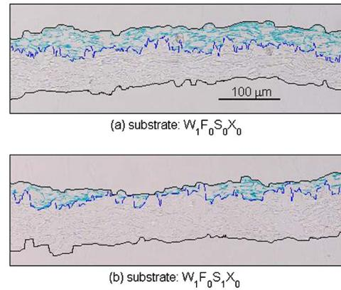
**Figure 2.** Image classifications for top and bottom surfaces of the paper sheets (solid lines) as well as interfaces of ink penetration (dashed lines). The samples are printed with (cyan) ink level 3 on hand sheets (a)  $W_1F_0S_0X_0$  and (b)  $W_1F_0S_1X_0$ , respectively.
