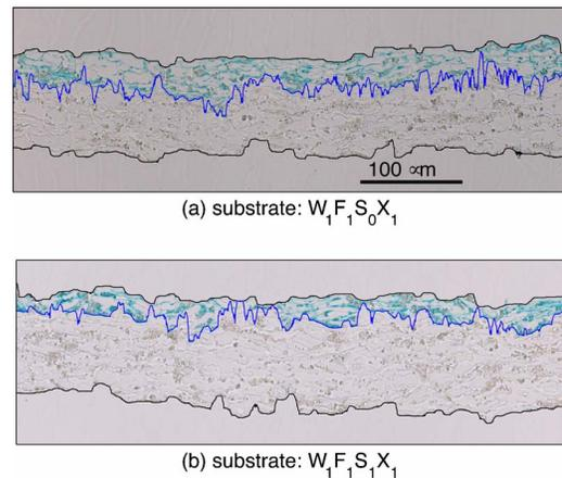
**Figure 3.** Dependence of ink penetration on paper composition. Two types of hand sheets,  $W_1F_1S_0X_1$  (in particular, with filler), and  $W_1F_1S_1X_1$  (containing both filler and internal size), are printed with ink cyan and ink level 3.
