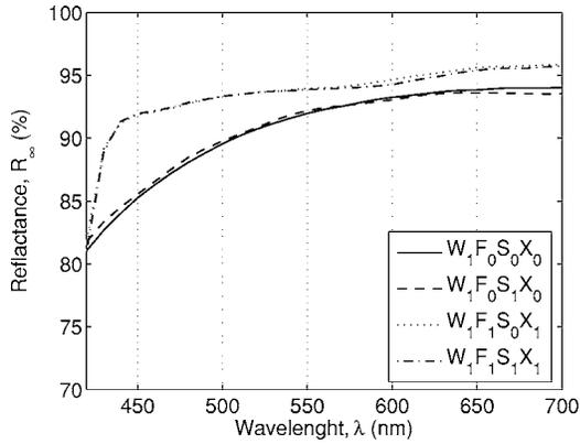
Figure 4. The spectral reflectance values of hand sheets (infinitely thick) of the four different material compositions namely  $W_1F_0S_0X_0$ ,  $W_1F_0S_1X_0$ ,  $W_1F_1S_0X_1$ , and  $W_1F_1S_1X_1$ .
