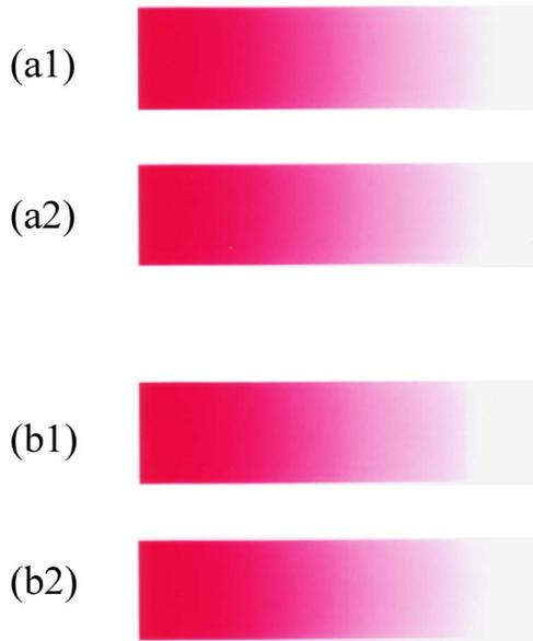
Figure 14. Printed gradation images. (a) Standard ink film: (a1) conventional density gradation method and (a2) highlight error diffusion method. (b) Nonstandard ink film: (b1) conventional density gradation method and (b2) highlight error diffusion method.
