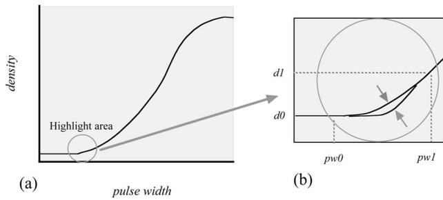
Figure 2. Density-tone curve of a dye sublimation transfer printing process.
