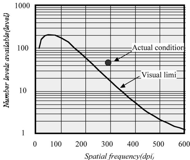
Figure 5. Spatial frequency response of human visual system by Roetling.
