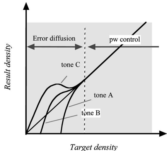
Figure 8. Result from a trial of highlight error diffusion method in a dye sublimation transfer printing process.
