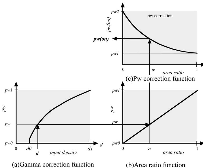
Figure 10. (a) Gamma correction function, (b) area ratio function, and (c)  $pw$  correction function.
