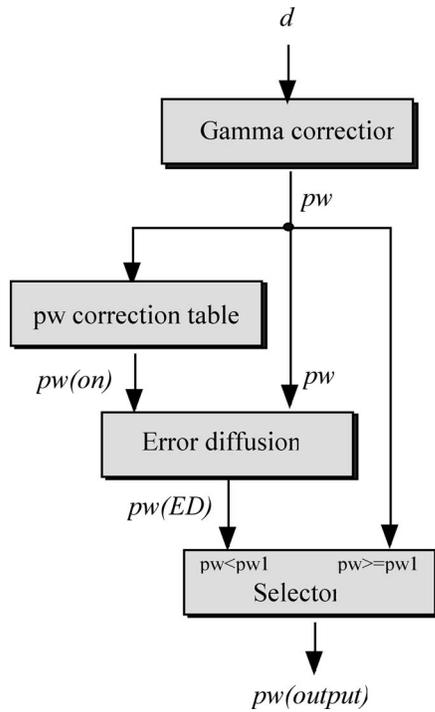
Figure 9. Proposed highlight error diffusion method.
