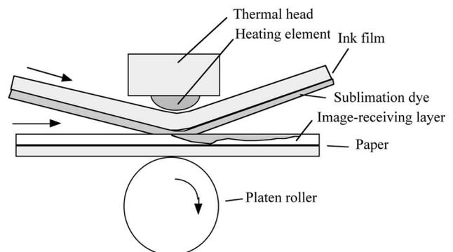
Figure 1. Printing process for dye sublimation transfer printing.
