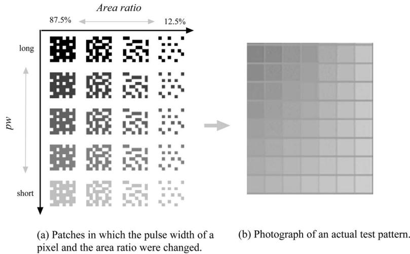
Figure 11. The printed test pattern. (a) Patches in which the pulse width of a pixel and the area ratio were changed. (b) Photograph of an actual test pattern.
