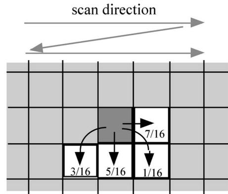
Figure 4. Floyd and Steinberg type error diffusion matrix.
