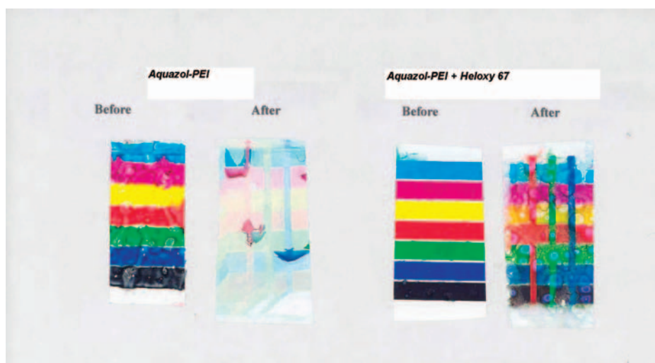
Figure 3. Comparative water submersion test results for uncrosslinked and crosslinked Aquazol®-PEI.
