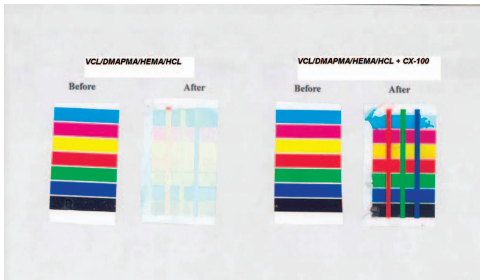
Figure 1. Comparative water submersion test results for uncrosslinked and crosslinked VCL/DMAPMA/HEMA/HCL.
