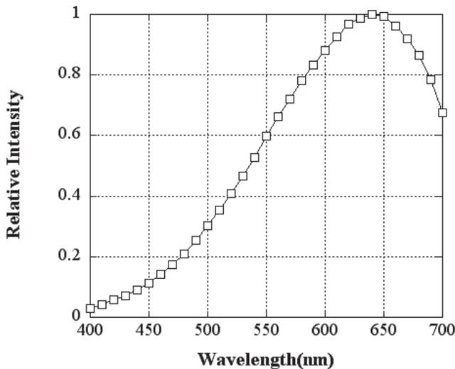
**Figure 2.** Spectral power distribution of the halogen lamp used for image capture.
