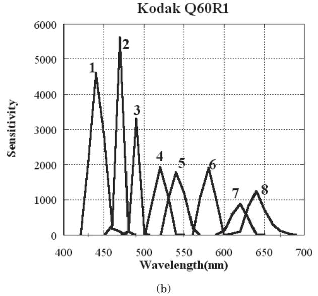
**Figure 1.** Spectral sensitivities of sensors used for the acquisition of the images of (a) Macbeth ColorChecker and (b) Kodak Q60R1.
