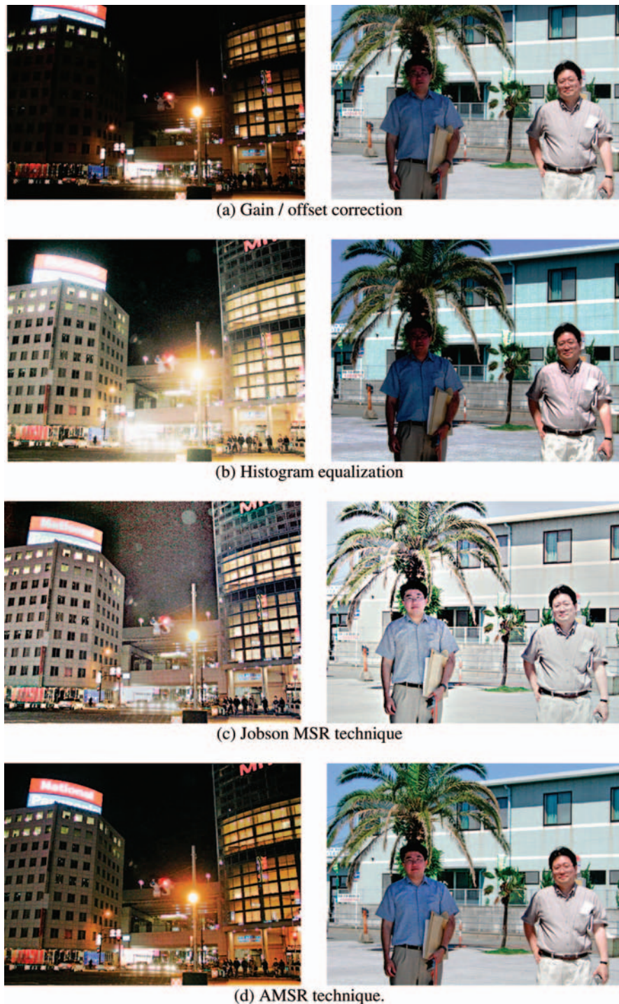
Figure 6. Output Images Processed by (a) Gain/Offset Correction; (b) Histogram Equalization; (c) Jobson MSR Technique; and (d) AMSR Technique.
