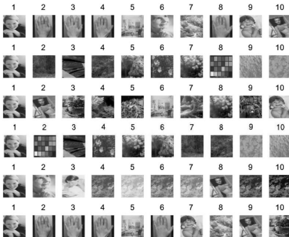
Figure 10. Ordered output for spectral images in the case of two-dimensional, spectral data-trained SOM. The distance measures used, row by row from top to down are: Euclidean distance, energy, Kullback–Leibler distance, maximum peak location, dynamic partial distance and Jeffrey divergence. Supplemental Material—Figure 10 can be found in color on the IS&T website ( www.imaging.org ) for a period of no less than two years from the date of publication.
