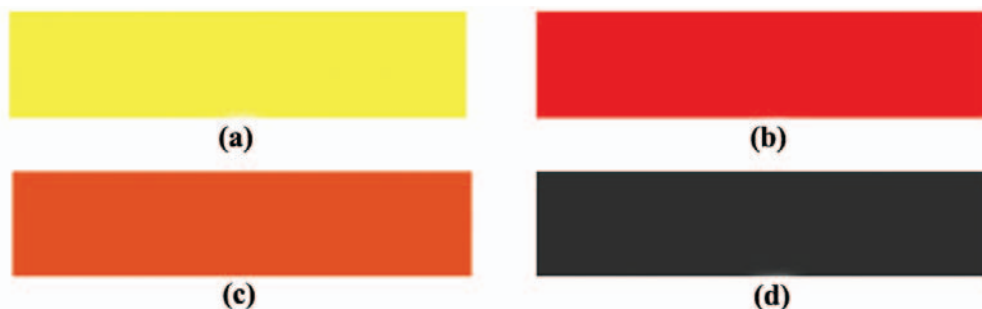
Figure 4. Color images of CLS coated in PVP (Photoshop simulations that best represented the transmission color observed). The colors are the result of changes in silver concentration.
