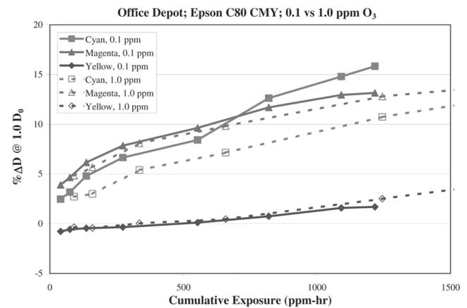
**Figure 16.** Comparison of the fade kinetics of the Epson C80 pure primary colors on the Office Depot Premium Photo Paper at 0.1 and 1.0 ppmv ozone.
