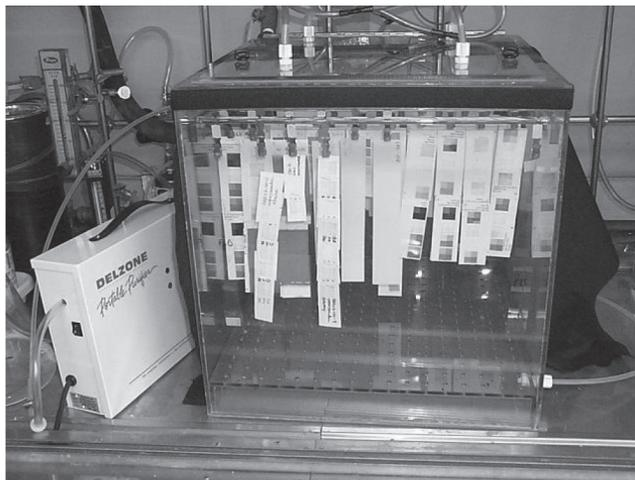
**Figure 1.** Photograph of an ozone chamber identical to those used for this study. The dark cloth that normally shrouds the entire chamber to prevent light-induced fade has been pulled back to provide a better view of the inside of the chamber.
