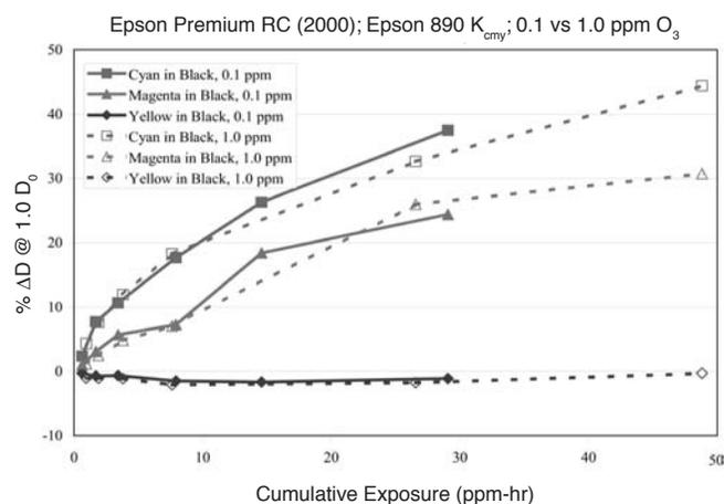
**Figure 9.** Comparison of the fade kinetics of the Epson 890 mixed primary colors on the Epson Premium RC Photo Paper (2000) at 0.1 and 1.0 ppmv ozone.
