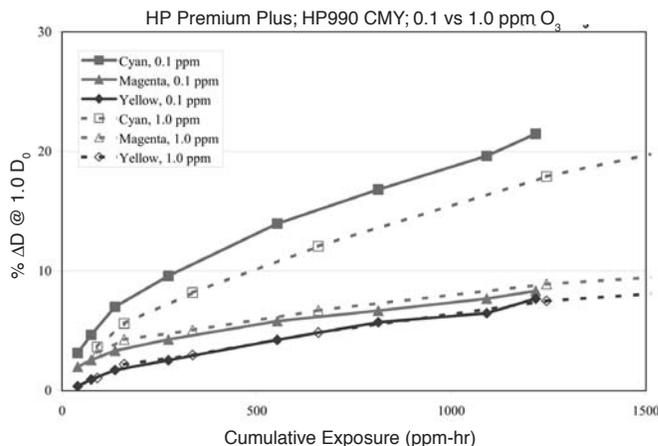
**Figure 12.** Comparison of the fade kinetics of the HP 990 pure primary colors on the HP Premium Plus Photo Paper at 0.1 and 1.0 ppmv ozone.
