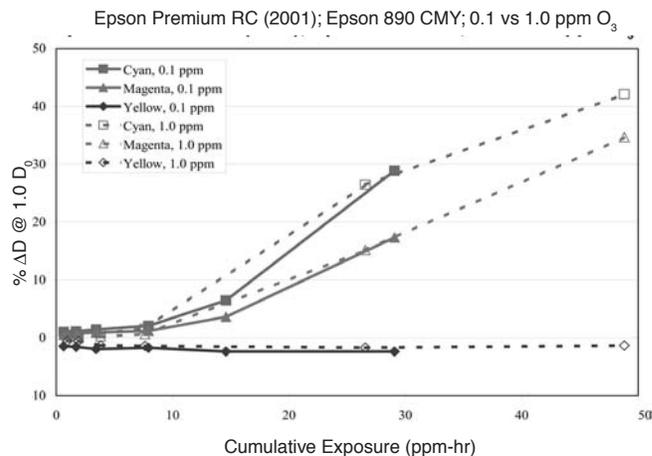
**Figure 8.** Comparison of the fade kinetics of the Epson 890 pure primary colors on the Epson Premium RC Photo Paper (2001) at 0.1 and 1.0 ppmv ozone.
