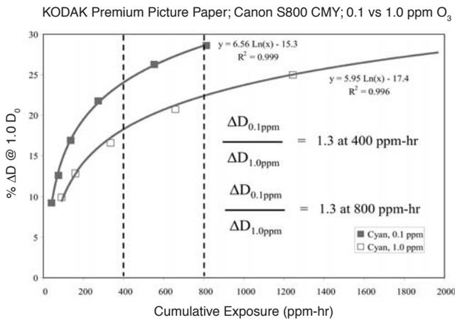
**Figure 14.** Comparison of the fade kinetics of the Canon S800 cyan ink patch on the KODAK Premium Picture Paper at 0.1 and 1.0 ppmv ozone illustrating the calculation of Rf.
