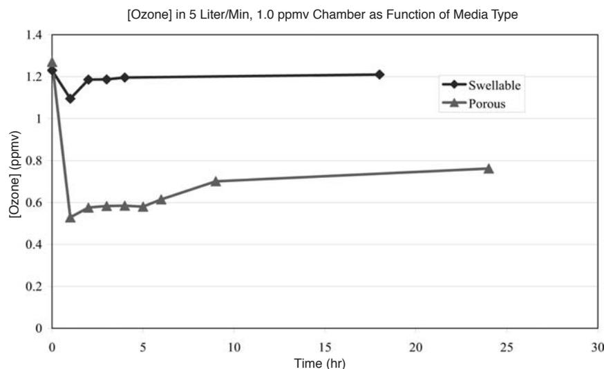
**Figure 6.** Aim versus measured ozone concentration after loading the chamber. Note that for this experiment, the target ozone concentration was 1.2 ppmv.
