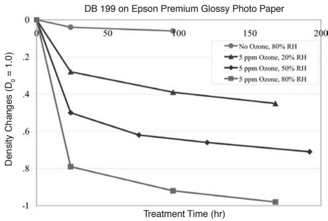
**Figure 2.** Effect of humidity on the ozone induced fade of a dye-based ink on a porous ink jet receiver.
