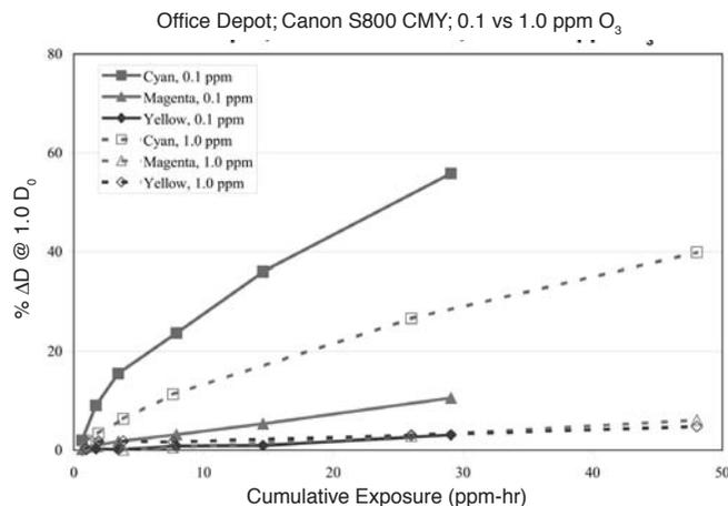
**Figure 10.** Comparison of the fade kinetics of the Canon S800 pure primary colors on the Office Depot Premium Photo Paper at 0.1 and 1.0 ppmv ozone.
