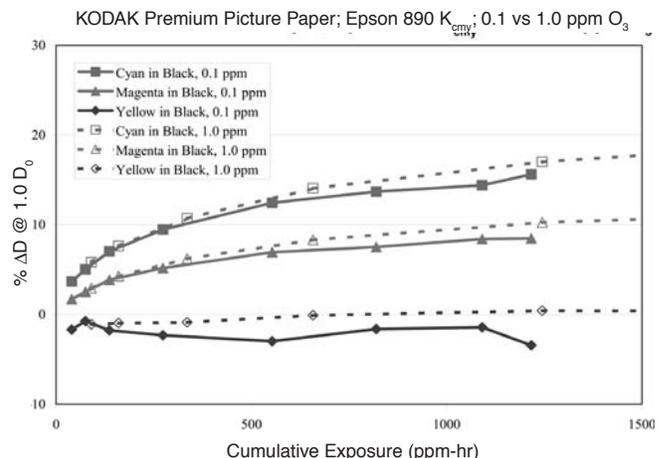
**Figure 13.** Comparison of the fade kinetics of the Epson 890 mixed primary colors on the KODAK Premium Picture Paper at 0.1 and 1.0 ppmv ozone.
