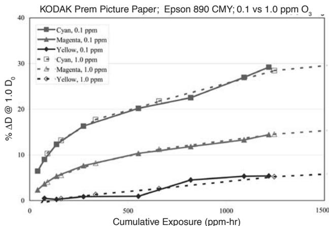
**Figure 11.** Comparison of the fade kinetics of the Epson 890 pure primary colors on the KODAK Premium Picture Paper at 0.1 and 1.0 ppmv ozone.
