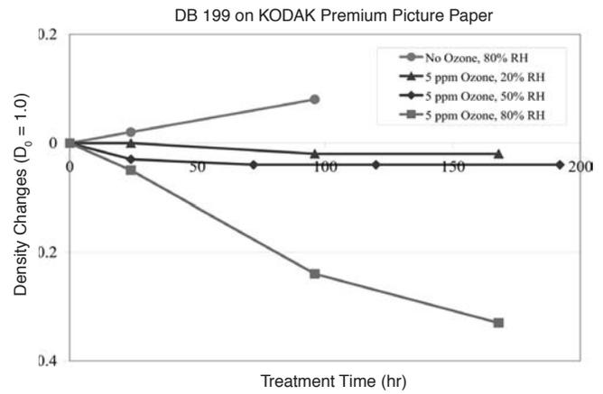
**Figure 3.** Effect of humidity on the ozone induced fade of dye-based ink on a swellable ink jet receiver.
