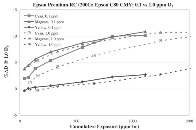
**Figure 15.** Comparison of the fade kinetics of the Epson C80 pure primary colors on the Epson Premium RC Photo Paper (2001) at 0.1 and 1.0 ppmv ozone.
