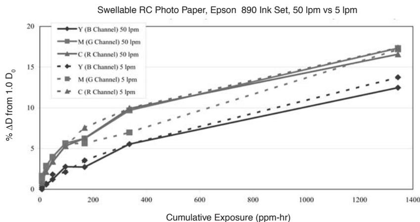
**Figure 5.** Effect of flow rate on the rate of fade of a swellable, slow fading system.
