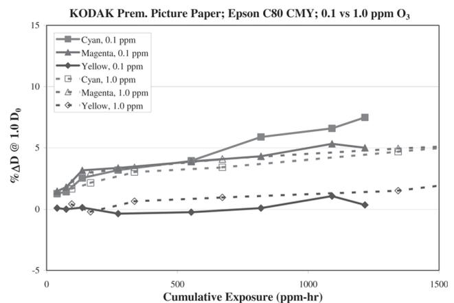
**Figure 17.** Comparison of the fade kinetics of the Epson C80 pure primary colors on the KODAK Premium Picture Paper at 0.1 and 1.0 ppmv ozone.
