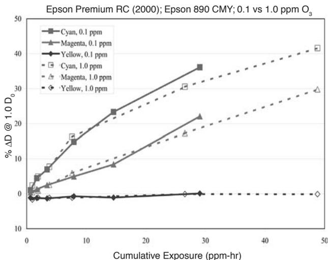
**Figure 7.** Comparison of the fade kinetics of the Epson 890 pure primary colors on the Epson Premium RC Photo Paper (2000) at 0.1 and 1.0 ppmv ozone.
