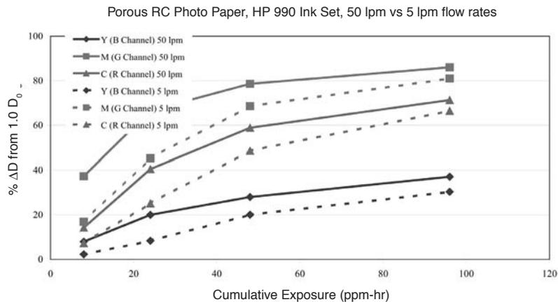
**Figure 4.** Effect of flow rate on the rate of fade of a porous, fast fading system.
