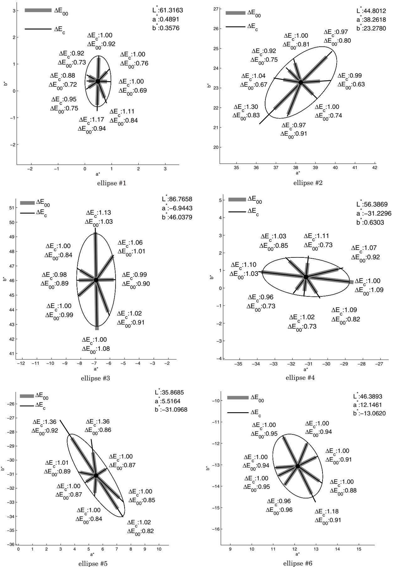
**Figure 16.** The ellipses showing the relative chromaticity differences assessed by this work and CIE DE2000 color difference formula (marked with wide black line and grey line and denoted as  $\Delta E_c$  and  $\Delta E_{00}$ , respectively).
