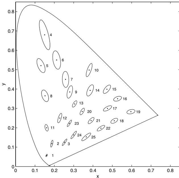
**Figure 1.** The MacAdam ellipses. The axes of plotted ellipses are 10 times their actual lengths.<sup>2</sup>
