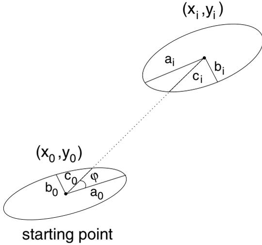
Figure 11. The visualization of the ellipse parameters.
