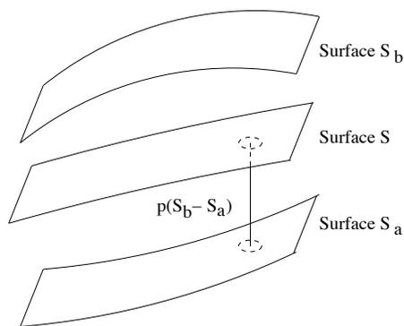
**Figure 4.** Defining surface  $S$  from the surfaces  $S_a$  and  $S_b$ . The distance between  $S_a$  and  $S$  is  $p(S_b - S_a)$ .
