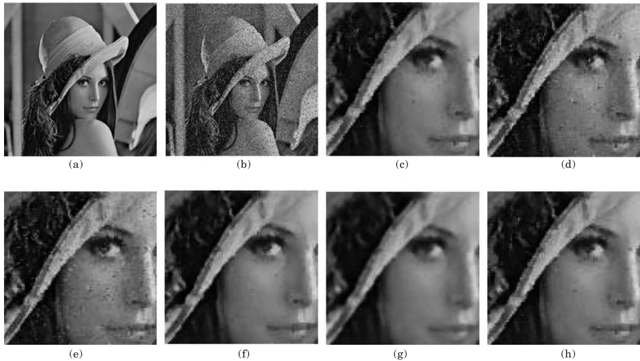
Figure 2. Subjective visual quantities of restored part of color image “Lena”, (a) original image; (b) input noisy image corrupted by 20% impulsive noise in each a channel; (c) AVMF filtered image; (d) VMF_FAS filtered image; (e) VWMKNNF filtered image (Simple) (f); VMMKNNF filtered image (Simple); (g) AMN-VMMKNNF filtered image; and (h) VMF filtered image. Supplemental Material—Figure 2 can be found in color on the IS&T website ( www.imaging.org ) for a period of no less than two years from the date of publication.
