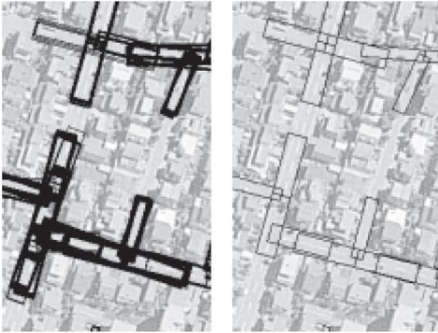
(a) Extracted intersections by thresholding (b) After overlap resolution
