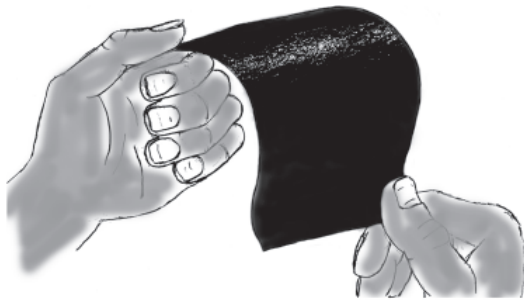
Figure 2. Illustration of an effective way of inspection when subjectively evaluating the gloss characteristics of a surface.
