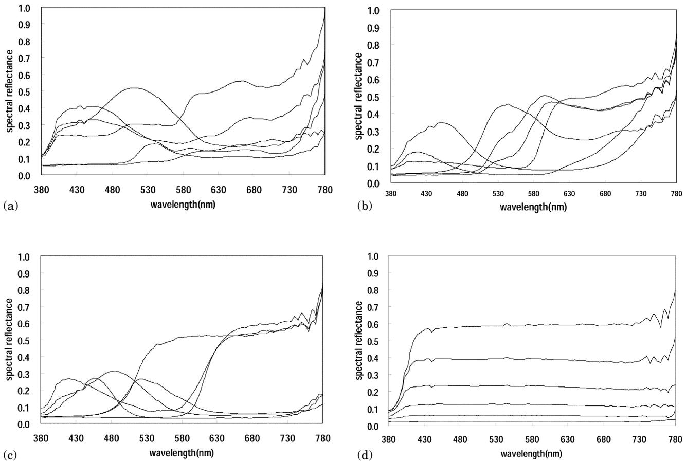
Figure 6. Measured spectral reflectance of 24 color patches of Gretag-Macbeth color checker.
