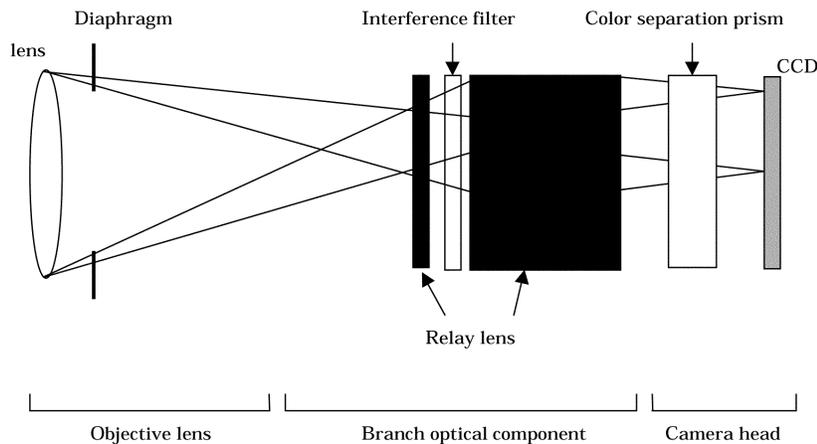
**Figure 13.** Schematic diagram of physical relationships of optical components
