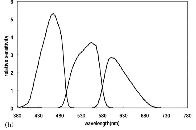
**Figure 5.** Measured spectral sensitivities of (a) six band camera system and (b) conventional HDTV camera.
