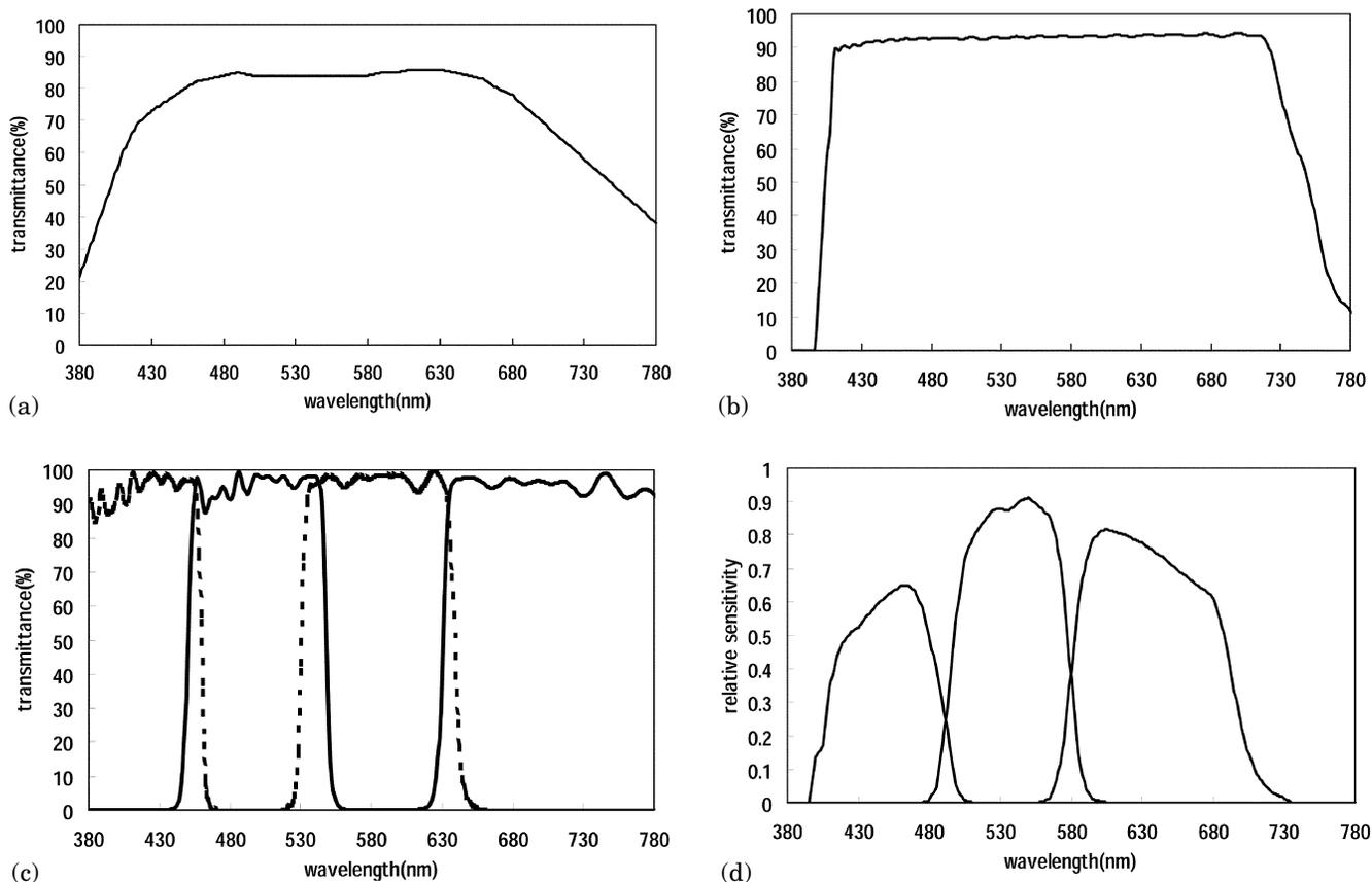
Figure 3. Spectral characteristics of optical components used in six band HDTV camera.
