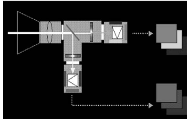
**Figure 2.** Principle of six band signal acquisition
