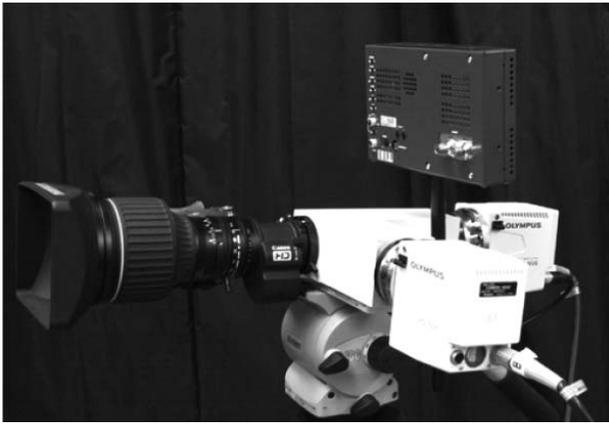
**Figure 1.** Appearance of six band HDTV camera
