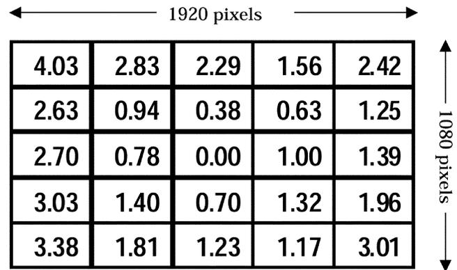
Figure 11. Color differences relative to color at center of imaging area.
