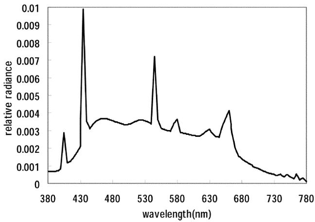
Figure 7. Spectrum of daylight
