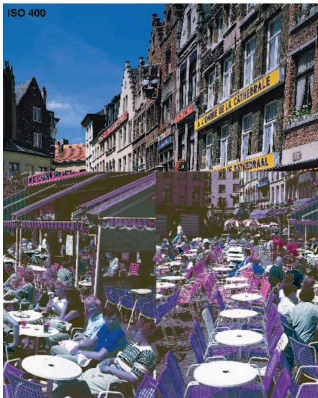
Color Plate 29. JPEG 2000 images produce typical “wavelet clouds” at higher compression rates (1:512). On the left is the original image, on the right the JPEG 2000 version. (Steingrímsson and Simon, pp. 572–585)
