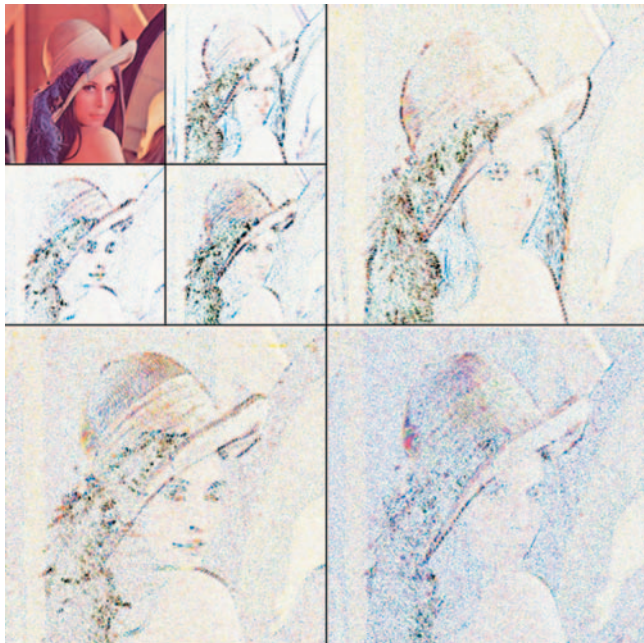
Color Plate 20. Original Lena image (top left) and its multiscale decompositions after one (top right), two (bottom left) and three (bottom right) decomposition steps using the biorthogonal 9/7 wavelet. ( Steingrímsson and Simon , pp. 572–585)
