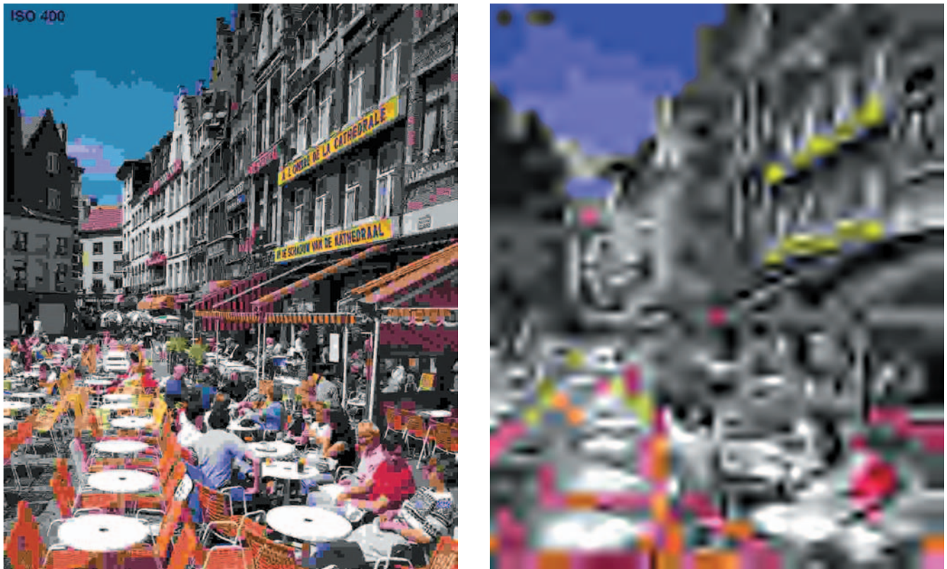
Color Plate 27. Test layout for quality comparisons: a JPEG (left) and a JPEG 2000 image (right) at random compression rates are confronted with each other. The examiner is now invited to select the image with fewer distortions with regard to the original. (Steingrímsson and Simon, pp. 572–585)
