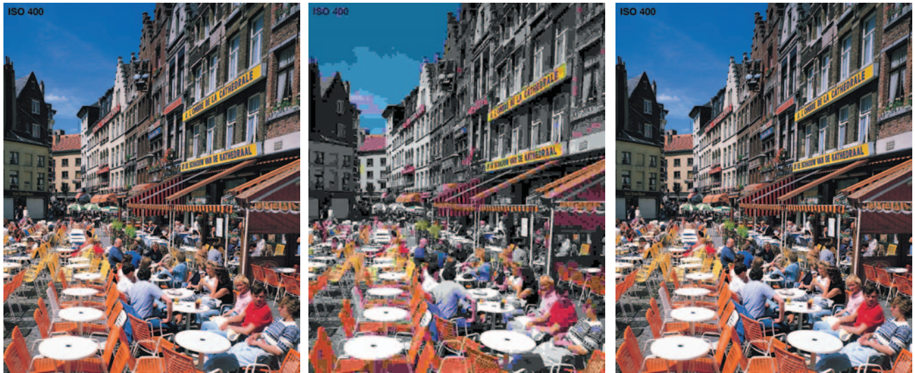
Color Plate 26. Test layout for identifying the compression limit of visually perceivable distortions. This test example contains a JPEG compression affected by heavy distortions (center image), surrounded by two original versions (left and right). (Steingrímsson and Simon, pp. 572–585)
