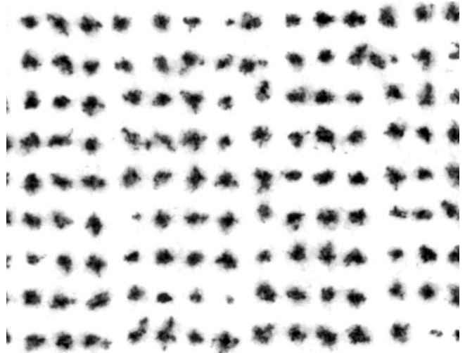
Figure 3. Black dot image for Epson printer on Weyerhaeuser paper.
