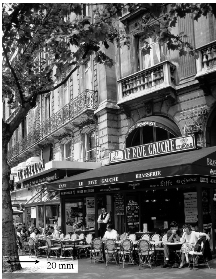
Figure 17. Printed sample using the newly developed multilayer thermoplastic resin based ink ribbon at 600 dpi.
