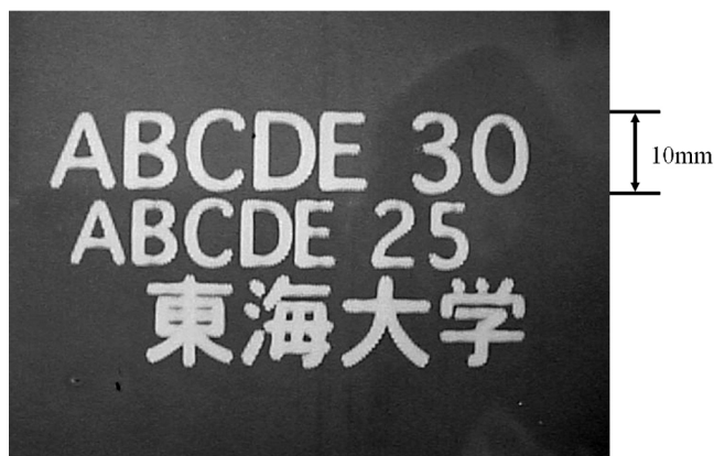
Figure 6. Typical image formed on liquid crystal medium by ion projection (LC type B, Composition ratio-50/50).
