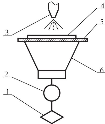
**Figure 1.** The sonic driver. 1 – signal generator, 2 – broadband (20 Hz – 22 kHz) amplifier, 3 – glass pipette tip, 4 – the print substrate, 5 – supporting table, 6 – transducer.
