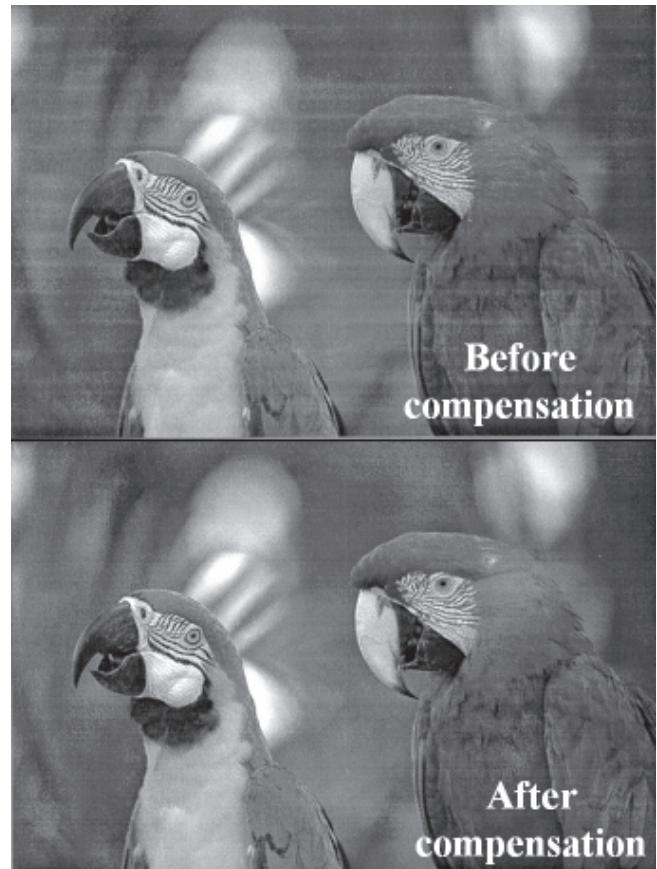
Figure 18. Actual printouts before and after compensation. Significant banding reduction can be seen in the bottom compensated image.
