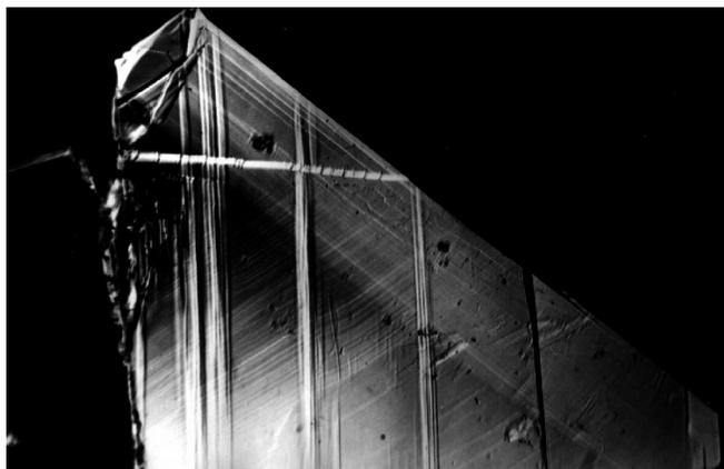
**Figure 3.** Optical micrograph of silver stearate single crystal during the first phase transition.
