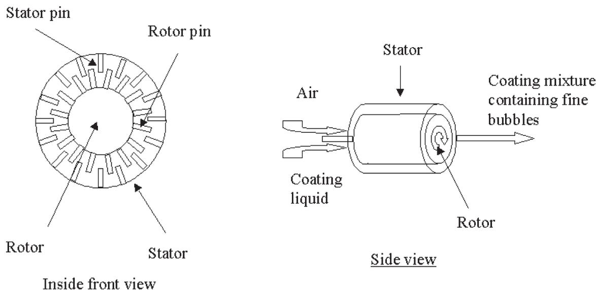
**Figure 1.** Schematic diagram showing a typical continuous whipping machine.
