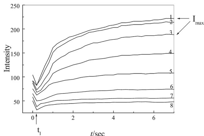
**Figure 6.** Developing process for each step on strip.  $I_{\max}$ : maximum intensity when development end;  $t_i$ : induction period.
