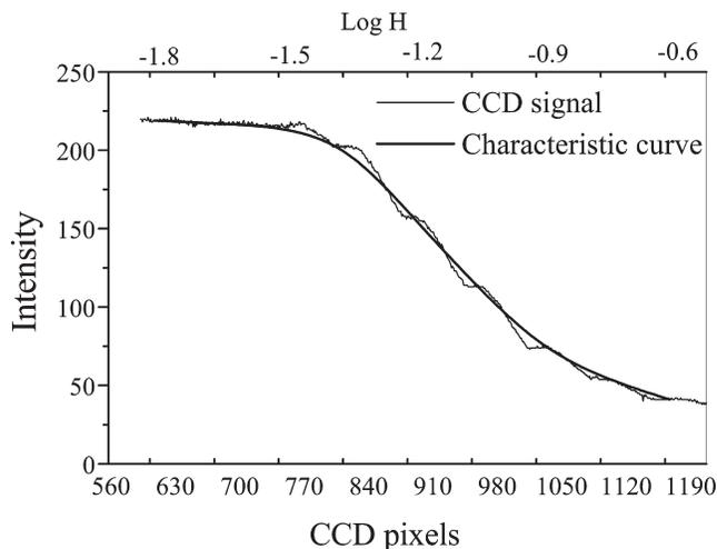
**Figure 5.** Relation between reflected light intensity of physically developed silver and CCD pixels (corresponding to exposure step) at development end.
