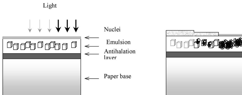
**Figure 2.** Cross sections of the experimental plate. a: Exposing; b: After development.
