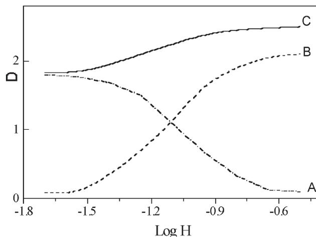
**Figure 1.** The theoretical characteristic curves for physical developed silver and chemical developed silver and the measured characteristic curve. A: physically developed silver; B: chemically developed silver; C: measured reflection density ( $D$ ) –  $\log E$ .
