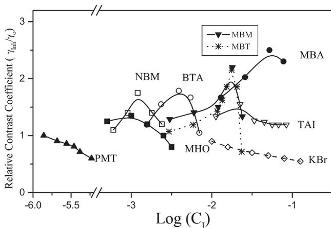
**Figure 8.** Effects of inhibitors on relative contrast coefficients at different concentrations  $C_i$ : concentration of inhibitor (mol/L).
