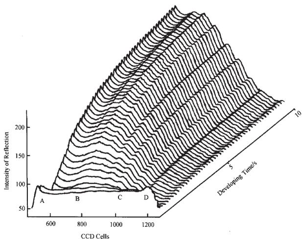
**Figure 4.** The three-dimension plot monitored by CCD—changes of reflection intensities with time and exposures. AB: weakly exposed steps; BC: moderately exposed steps; CD: strongly exposed steps.
