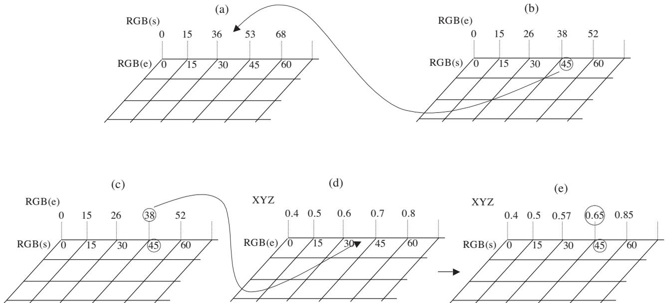
**Figure 3.** (a) It is possible to construct a lookup table between 'exposure' and 'scanned' RGB. This lookup table can be inverted (b). Concatenation of the inverted lookup table (c) with the XYZ lookup table (d) provides the final input profile lookup table (e).
