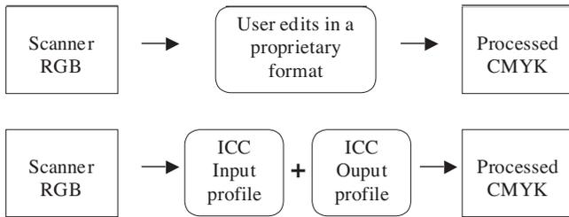
**Figure 1.** The aim of the current work is to replace a proprietary edit file with an ICC input and output profile.
