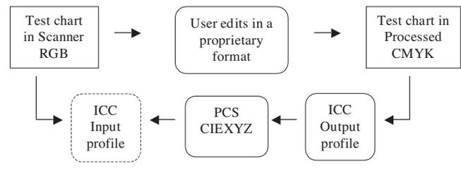
**Figure 2.** A test chart is processed to CMYK via the proprietary edit file. The CMYK patch values are converted via an output profile to XYZ. A new input profile is made between the RGB scan of the test chart and the new XYZ values.
