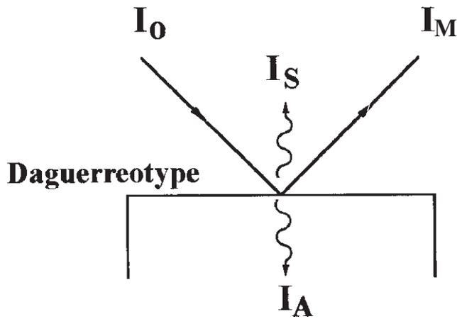
**Figure 1.** Schematic of the energy balance of light specular and diffuse reflected, and absorbed on a Daguerreotype surface.
