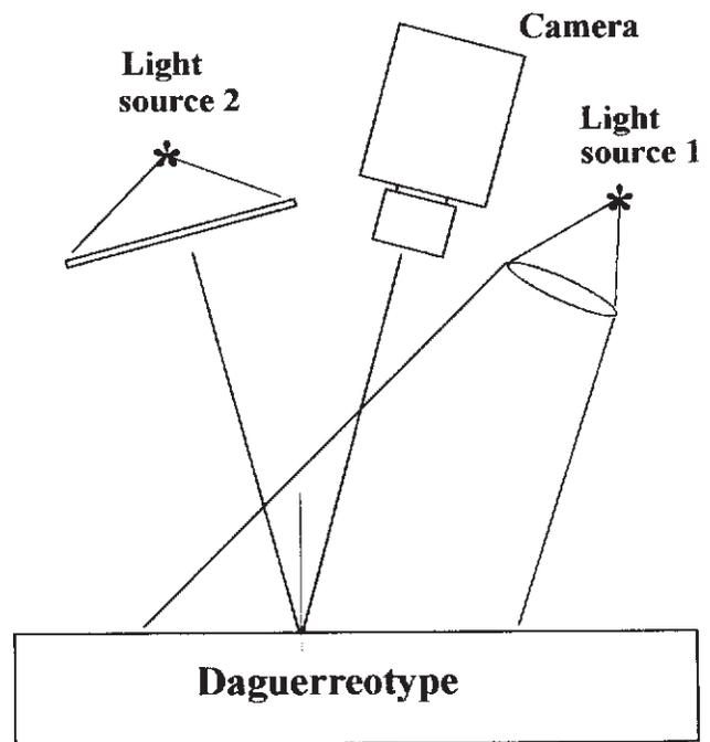
**Figure 2.** Experimental setup for capturing positive and negative images of a Daguerreotype. Source 1 provides a collimated light beam such that only the scattered light component can be viewed by a camera or observer. Illumination of the Daguerreotype by Source 1 produces a positive image. Source 2 is a white screen placed in a position where its reflection by a Daguerreotype plate can be viewed by the camera or observer. Therefore, Source 2 creates a negative image of the Daguerreotype.
