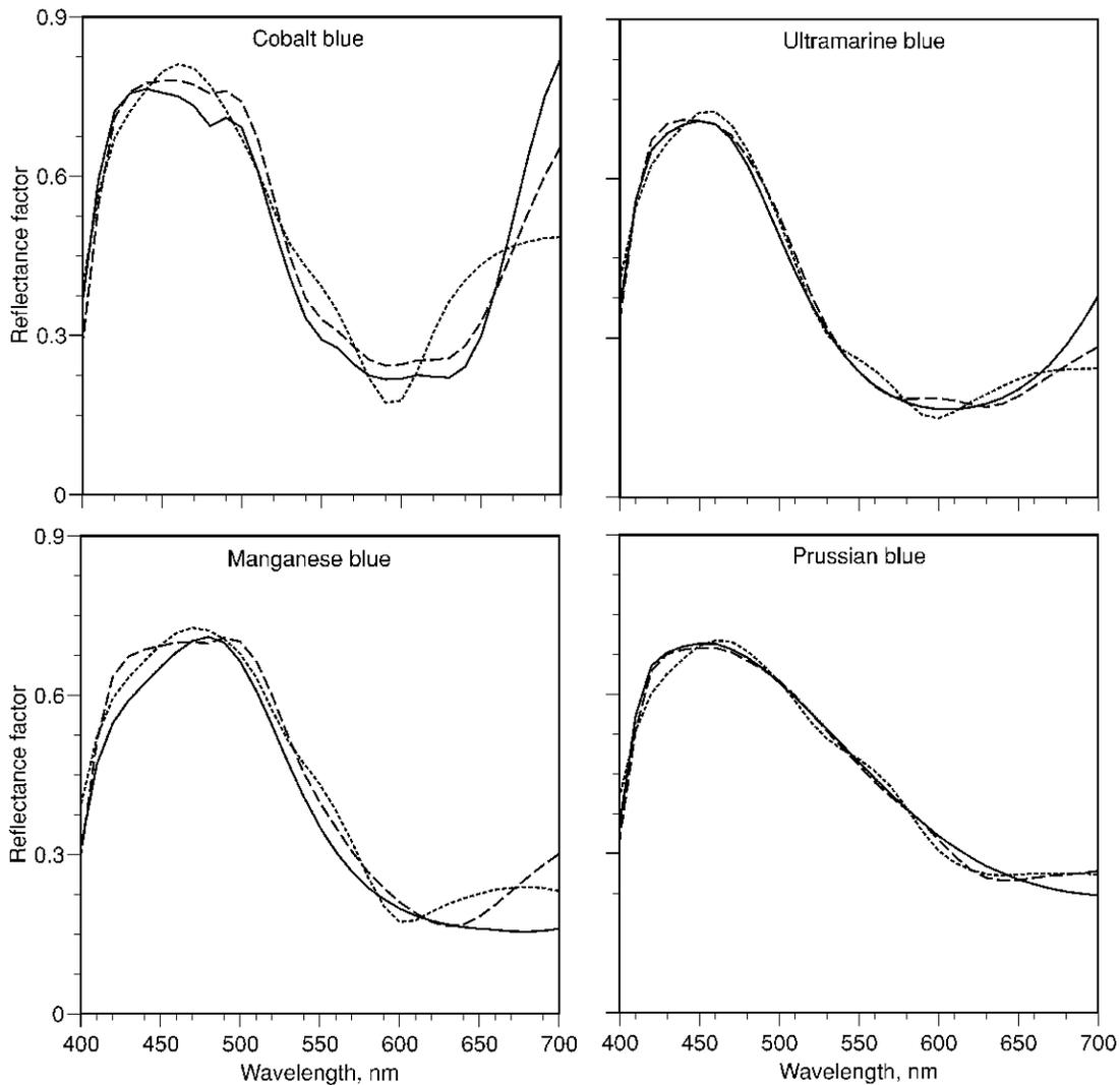
**Figure 27.** Spectral estimation of four samples from the artist oil target shown in Fig. 23: measured, solid line, estimated from spectral data of ColorChecker, dotted line, estimated from spectral data of the entire target, dashed line.
