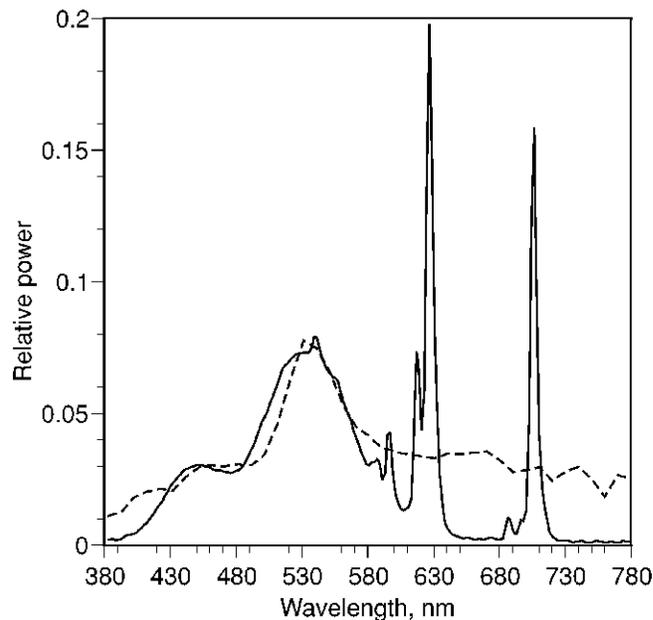
**Figure 2.** Spectral properties of a metamer pair formed by foliage, illuminated by natural daylight (dashed line), and a CRT display (solid line).<sup>6</sup>
