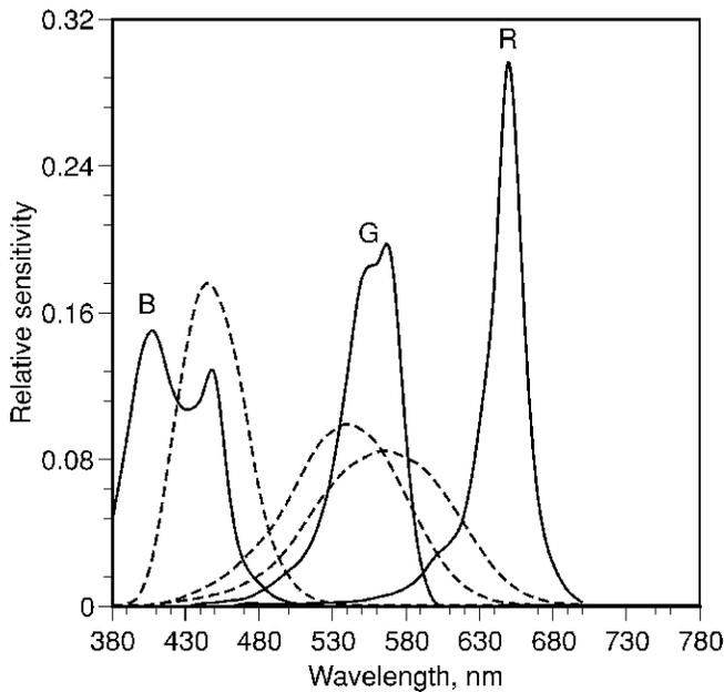
**Figure 9.** Spectral sensitivities of typical transparency film (solid lines), in this case Eastman Kodak Ektachrome 64T.<sup>15</sup> The human visual system's spectral sensitivities, shown in Fig. 1, are also plotted (dashed lines).
