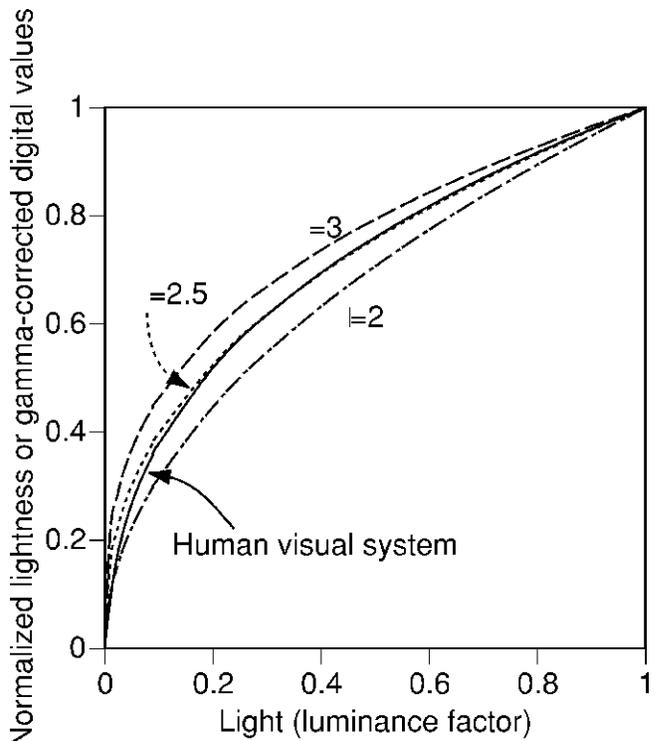
**Figure 19.** Relationship between light, expressed as luminance factor, and lightness (solid line) or gamma-corrected signals ( $\gamma=3$ : dashed line;  $\gamma=2.5$ : dotted line;  $\gamma=2$ : dot-dashed line).
