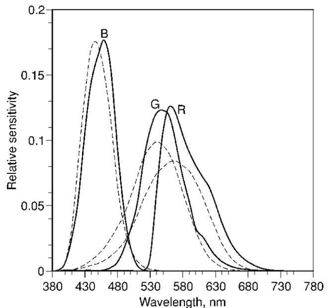
**Figure 8.** Spectral sensitivities of a monochrome scanback with three optimized color filters (solid lines), normalized to equal area. These sensitivities include the CCD spectral sensitivity, filter transmittances, and infrared radiation blocking filter. The human visual system's spectral sensitivities, shown in Fig. 1, are also plotted (dashed lines).
