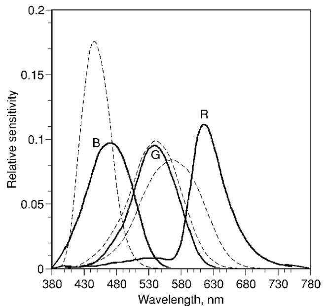
**Figure 7.** Spectral sensitivities of a typical color CCD two-dimensional array (solid lines), normalized to equal area. These sensitivities include the CCD spectral sensitivity, filter transmittances, and infrared radiation blocking filter. The human visual system's spectral sensitivities, shown in Fig. 1, are also plotted (dashed lines).
