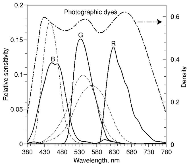
**Figure 6.** Spectral sensitivities of a typical scanback (solid lines), normalized to equal area. These sensitivities include the CCD spectral sensitivity, filter transmittances, and infrared radiation blocking filter. The human visual system's spectral sensitivities, shown in Fig. 1, are also plotted (dashed lines) as is the spectral density of typical photographic dyes combined to reproduce a medium-gray color (dashed-dotted line).
