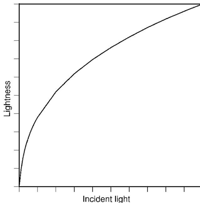
Figure 5. Nonlinear response between incident light and lightness. The incident light can have units of radiance, irradiance, luminance, illuminance, or simply power per unit area. (CIE  $L^*$  is used as a representation of lightness.)
