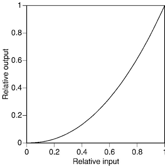
**Figure 11.** CRT nonlinearity. This nonlinearity is inherent to all vacuum tubes.<sup>20,21</sup>
