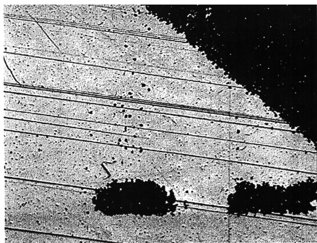
Onset of "N" image degradation 30 nN Tangential force on toner particles Surface treated toner 1.0% silica / 0.35% titania
