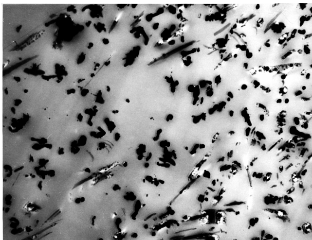
Figure 4. Transmission electron micrographs of sample corresponding to curve 1 in Fig. 3. with (left) and without (right) pre-exposure heating (10 s at 115°C), after development for 10 s at 115°C (60,000X).
