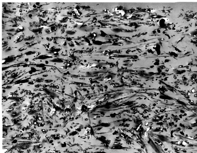
Figure 4. Transmission electron micrographs of sample corresponding to curve 1 in Fig. 3. with (left) and without (right) pre-exposure heating (10 s at 115°C), after development for 10 s at 115°C (60,000X).
