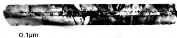
Figure 2. Cross-section image of AgBrI platelet showing the existence of internal (111) twin boundaries. Secondary twin boundaries occasionally found in the upper (or lower) primary twin regions. They have now been detected in the middle twin region.
