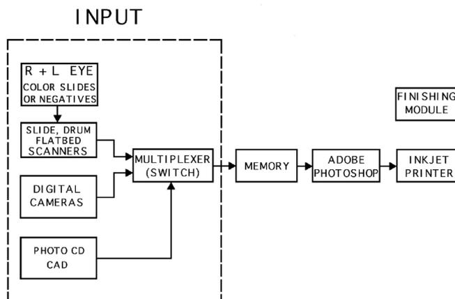
**Figure 4.** Flow diagram illustrating the preparation of digitized stereoscopic polarizing images. The principal steps are: (1) the preparation of a digitized left–right image pair, (2) storage of the two images as a left–right image file, (3) paste-layering, using Adobe Photoshop. Following adjustment of contrast and color, suitable cropping, and stereo registration, the two images are printed sequentially, one on each surface of the two-sided sheet.
