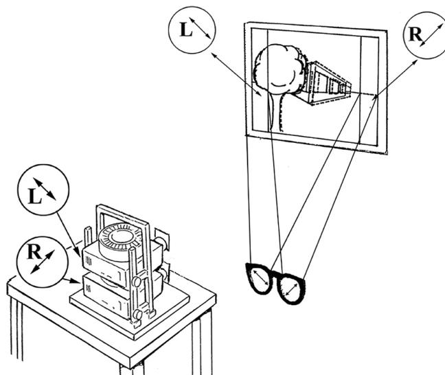
Figure 1. 3-D projection display with two projectors.
