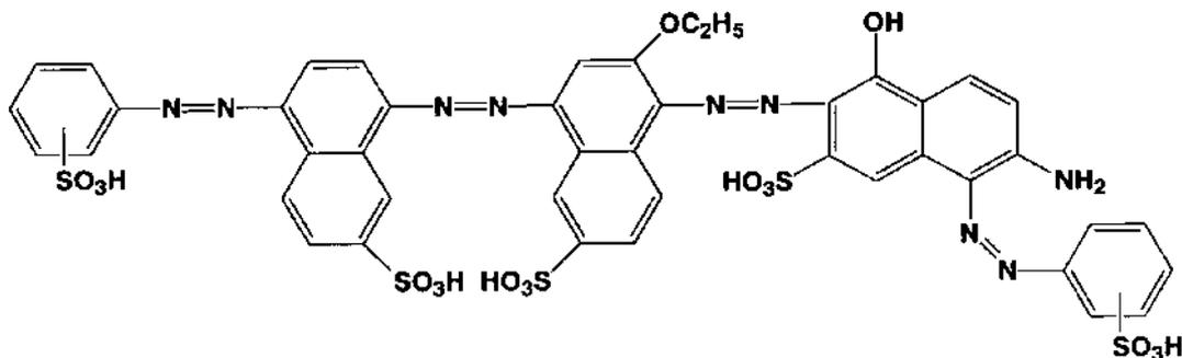
Figure 6. A typical dichroic image dye, Direct Green 27.
