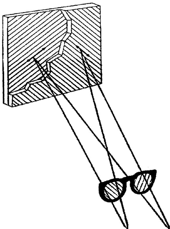
**Figure 2.** The Vectograph concept, using paired, oppositely oriented polarizing images.
