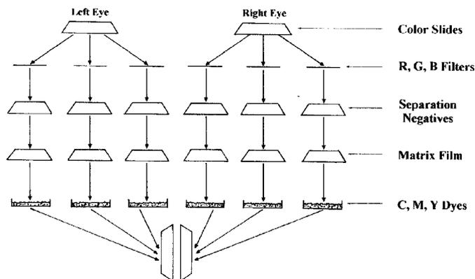
**Figure 3.** Color Vectograph image printing by dye-transfer process.
