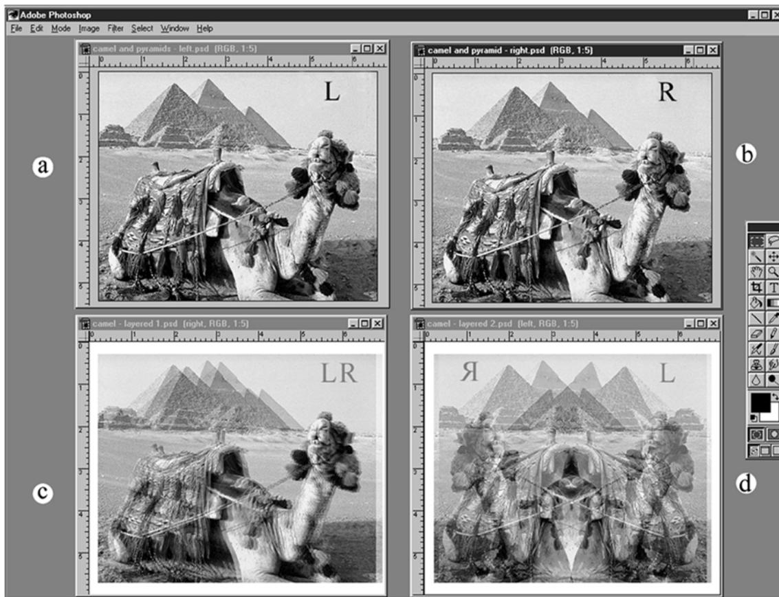
Figure 5. Monitor screen views showing the steps in stereoscopic registration of image pair.
