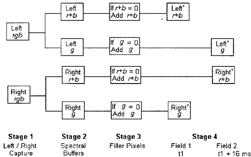
**Figure 4.** Stages of spectral multiplexing. In Stage 1,  $r, g, b$  image pixels are captured and in Stage 2, pixels are separated into a magenta buffer ( $r + b$ ) and a green buffer ( $g$ ) for the left and right images. In Stage 3, filler pixels are added so pure red, green, blue, or magenta areas of the image will not be dark during the alternate field. Stage 4 shows the field-sequential presentation of left and right images.
