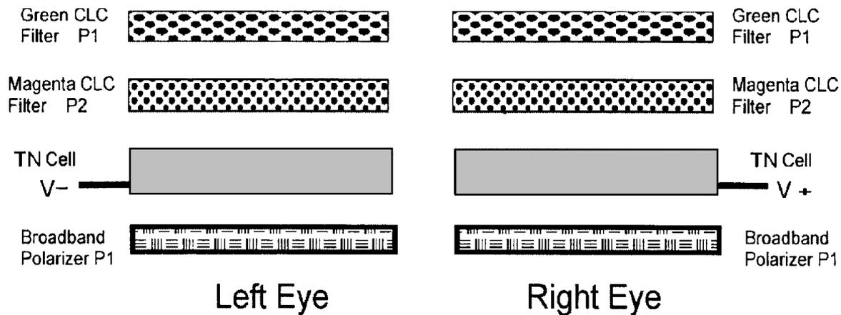
**Figure 5.** Eyewear for spectral demultiplexing. Left and right eye optics are identical: shown in order from the image back to the eye are green cholesteric liquid crystal filters in a P1 state, magenta cholesteric liquid crystal filters in a P2 state, active TN cells, and a broadband polarizer (analyzer) in a P1 state. The TN cells are shown in a state to transmit the Field 1 image; to transmit the Field 2 image, the voltage polarities are reversed.
