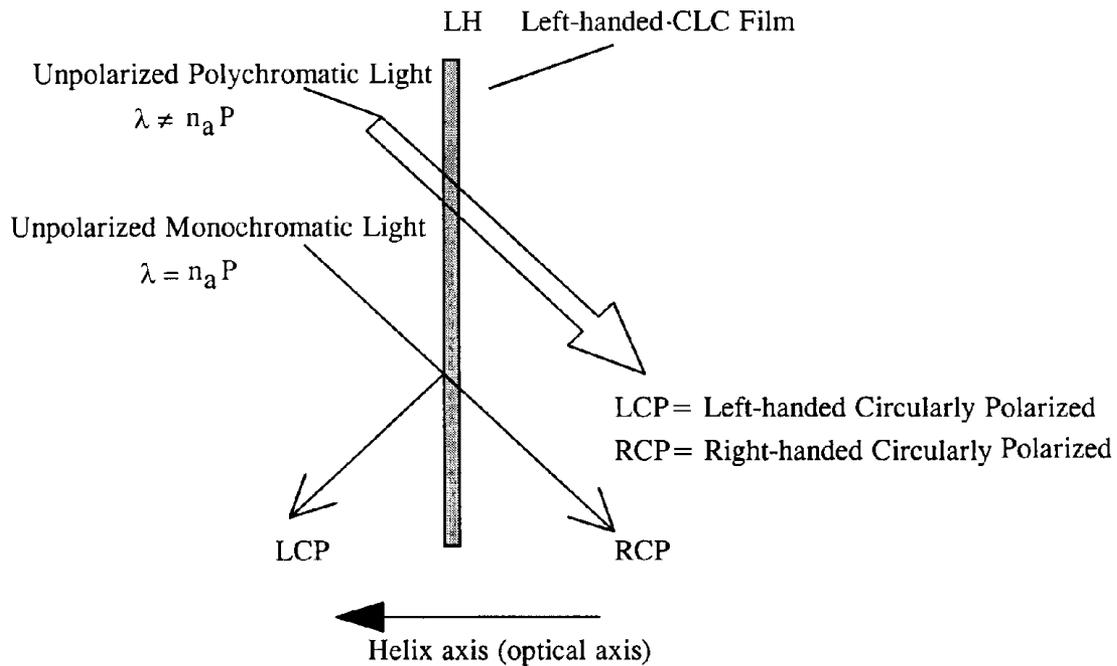
**Figure 6.** Reflective properties of left-handed CLC. The wavelength of light reflected is determined by the pitch of the CLC, and the direction of polarization, RCP or LCP, is determined by the direction of helical twist of the CLC.
