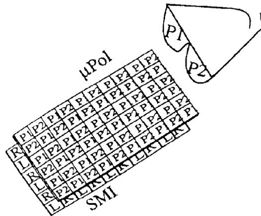
**Figure 3.** Demultiplexing a spatially multiplexed image (SMI). Right image pixels are aligned with the P1 elements of the  $\mu$ Pol array, left image pixels with P2 elements. Through cross-polarization, only the right image pixels are transmitted through the polarized lenses to the right eye and left image pixels to the left eye.
