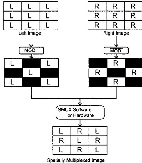
**Figure 2.** Spatial multiplexing. Images from digital sources are multiplexed with software, images from video sources are multiplexed with field-switching hardware, and photographic images can be multiplexed using the  $\mu$ Pol array self-aligned to the film for both multiplexing and demultiplexing. Two-dimensional multiplexing is shown.
