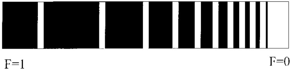
**Figure 13.** Illustration of a halftone line pattern that is FM in terms of the spaces between the lines, but AM with respect to the lines.
