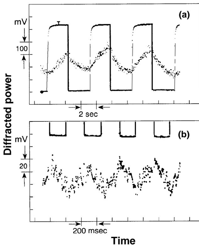
**Figure 3.** Modulation of holographic gratings (dotted traces) as a result of square wave modulation of UV beam (line traces). The modulated gratings were continuously exposed to the recording beams, each of  $20 \text{ mW/cm}^2$ , (a) with modulation frequency of 0.2 Hz, (b) with 2.5 Hz.
