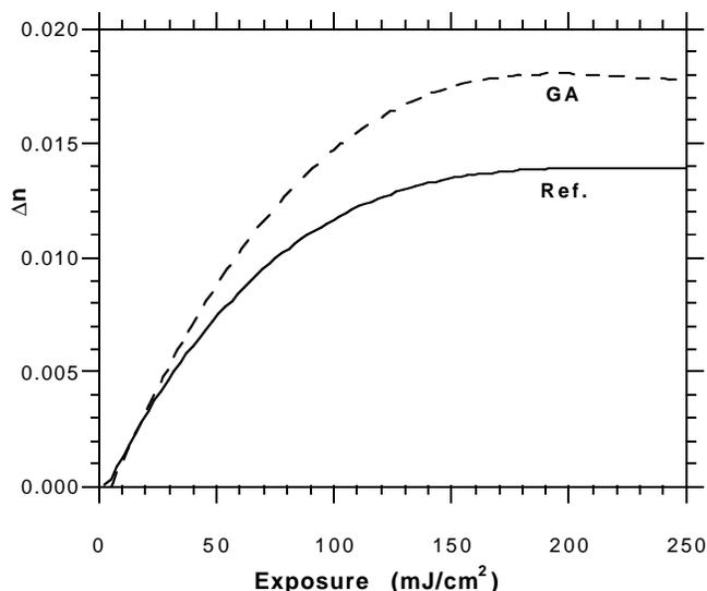
**Figure 12.** Calculated refractive index modulation as a function of exposure derived from data of Fig. 11 and using Eq. 9.
