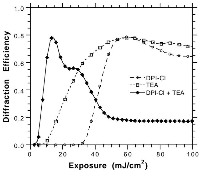
**Figure 7.** DE versus exposure of holographic gratings recorded at 514 nm in PVA-acrylamide photopolymers sensitized by eosin Y and different charge transfer agents: squares—TEA alone, circles—DPI-Cl alone; diamonds—TEA and DPI-Cl. Formulations are according to Table I.
