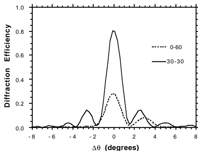
**Figure 13.** DE as a function of angular deviation from Bragg conditions of holographic gratings recorded in photoactive polymer layers with unslated (30-30) and slanted (0-60) fringe orientation.
