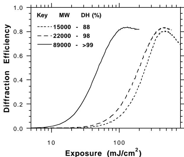
**Figure 10.** Diffraction efficiency versus exposure of holographic gratings recorded in photopolymer layers with PVA binders for different molecular weights (MW) and degrees of hydrolysis (DH).
