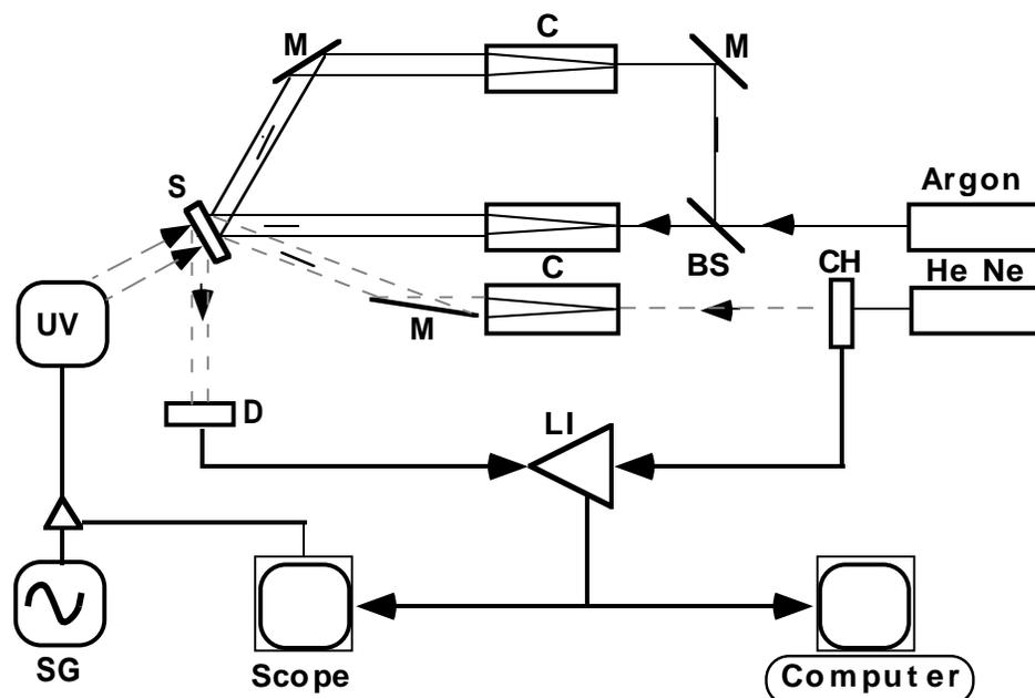
**Figure 1.** Schematic of the optics setup for holographic recording and readout: SG—signal generator, UV—mercury lamp, D—Si photodetector, S—sample, M—mirror, C—collimators and spatial light filters, BS—beamsplitter, CH—chopper.
