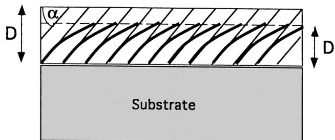
**Figure 14.** Schematic representation for the effect of nonlinear shrinkage in holographic gratings recorded in photoactive polymer layers.
