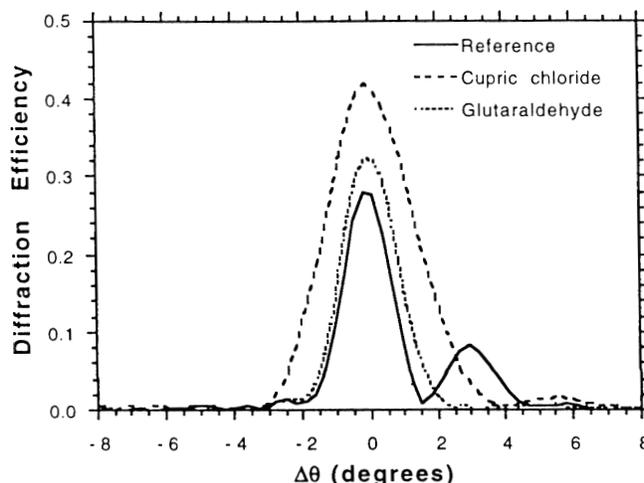
**Figure 15.** DE versus angular deviation from Bragg conditions for holographic gratings recorded with slanted fringe orientation in photoactive polymer layers with or without crosslinking agents.
