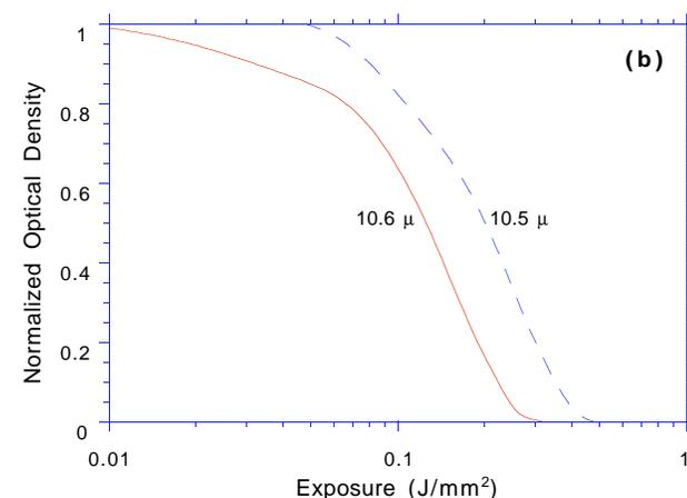
**Figure 5.** Normalized optical density as a function of absorbed IR exposure energy of spiropyran-MMA copolymer layers. The irradiation wavelengths were 10.6 and 10.5  $\mu\text{m}$  from a  $\text{CO}_2$  laser. (a) the spiropyran concentration is 6 mol %. (b) The spiropyran concentration is 25 mol %.
