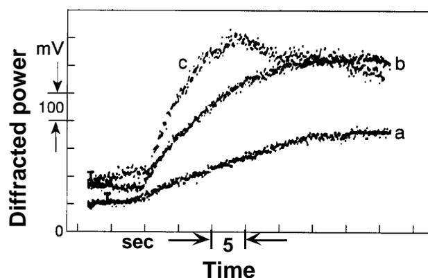
**Figure 4.** Temporal holographic growth in spirooxazine/PMMA for different recording beam intensities: (a)  $10 \text{ mW/cm}^2$ , (b)  $20 \text{ mW/cm}^2$ , (c)  $40 \text{ mW/cm}^2$ . The UV excitation beam intensity was  $10 \text{ mW/cm}^2$ .
