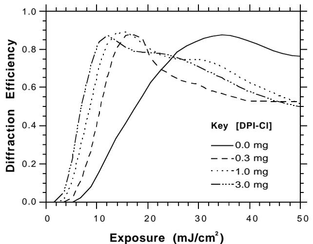
**Figure 8.** Diffraction efficiency versus exposure for different DPI-Cl concentrations and constant TEA concentration. Other parameters as for holographic grating of Fig. 7.
