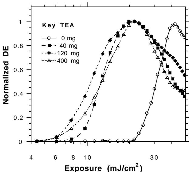
**Figure 9.** Normalized diffraction efficiency versus exposure for different TEA concentrations and constant DPI-Cl concentration. Other parameters are the same as for holographic gratings of Fig. 7.
