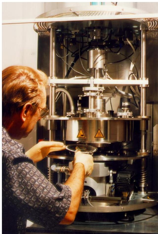
**Figure 3.** Hot stamping press at PSI for the replication of DOEs in polycarbonate foil.
