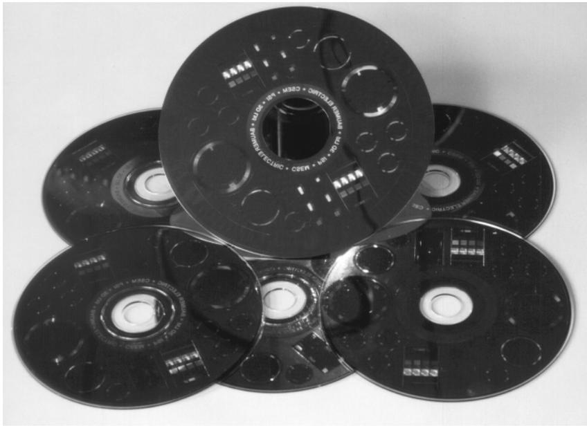
**Figure 10.** Ni stamper (master) and injection molded CDs with test DOE microstructures.
