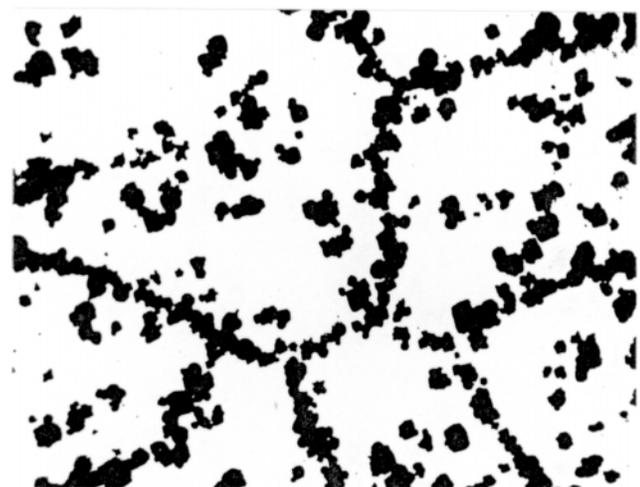
**Figure 26.** Development centers formed at sites of termination of dislocations of the polyhedral subboundaries in a thin sheet AgCl crystal sensitized with a solution of  $\text{Na}_2\text{S}_2\text{O}_3$  (X 1,725).<sup>6</sup>
