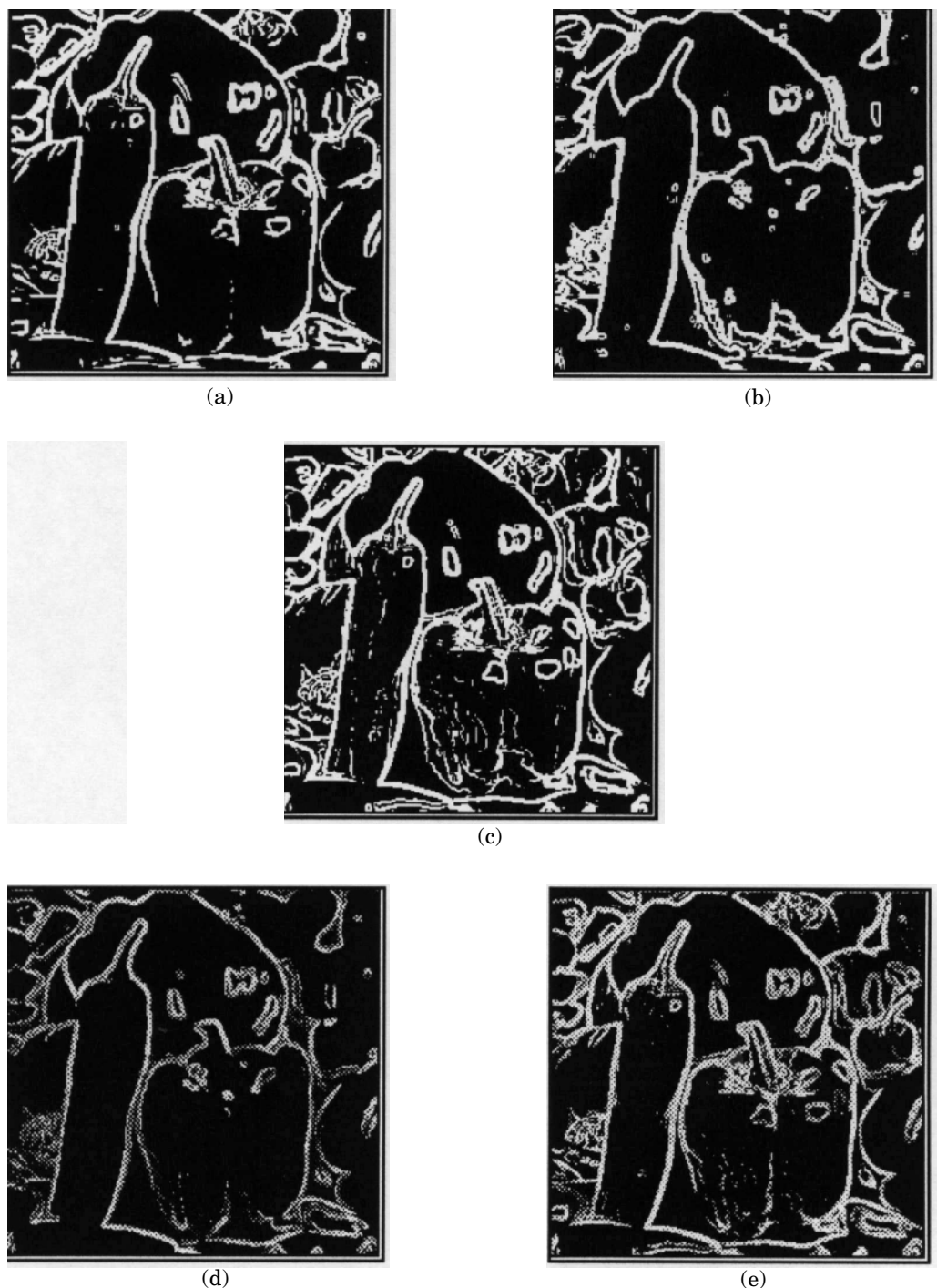
Figure 15. (a) Edge elements detected in Fig. 1(a); (b) edge elements detected in Fig. 1(b); (c) edge elements detected in Fig. 1(c); (d) color edge differences between Fig. 15(a) and Fig. 15(b); (e) color edge differences between Fig. 15(a) and Fig. 15(c). In Figs. 15(d) and 15(e), white pixels correspond to color edge differences equal to zero.
