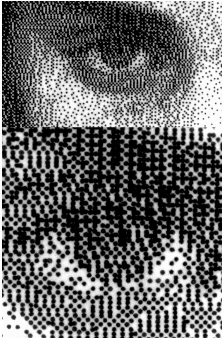
Figure 11. Photomicrograph of fixed spot printing using the same printhead and original image as was used in Fig. 10.
