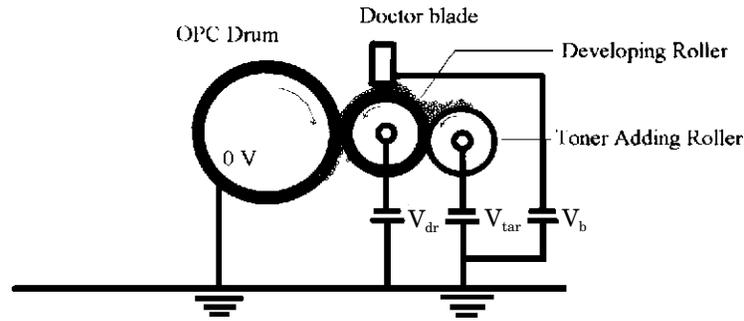
Figure 1. Schematic of the experimental development system.
