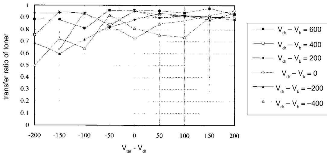
Figure 8. Transfer ratio under different dc bias voltages.
