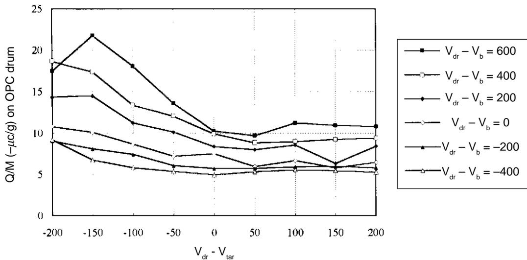
Figure 7. Q/M on OPC drum.
