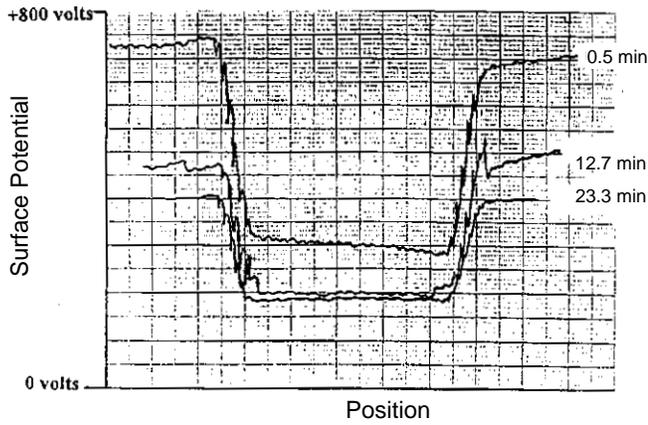
**Figure 1.** The electrostatic image structure of a positive charging photoreceptor at 0.5-, 12.7-, and 23.3-min delays after exposure through a 0.25-cm slit. The position axis units are 0.0255 cm/major division.
