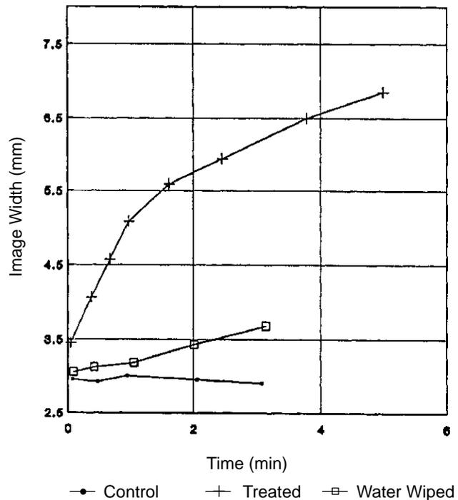
**Figure 4.** The square well image width, as a function of delay after exposure through a 0.25-cm slit, for a positive charging photoreceptor before and after spraying the surface with a commercially available glass cleaner. The treated photoreceptor is returned to the original state by rinsing the surface with water.
