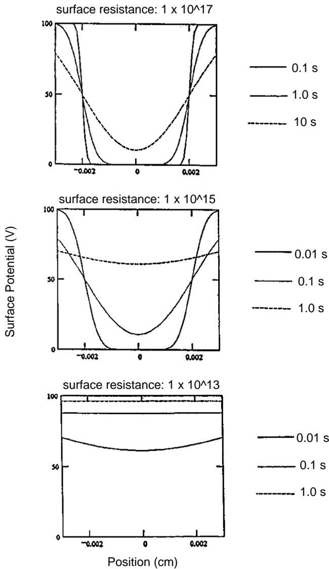
**Figure 5.** Calculated 40- $\mu\text{m}$  square-well image shapes on a 20- $\mu\text{m}$  photoreceptor as a function of time after exposure for surface resistances of  $1 \times 10^{17}$ ,  $1 \times 10^{15}$ , and  $1 \times 10^{13} \Omega$ .
