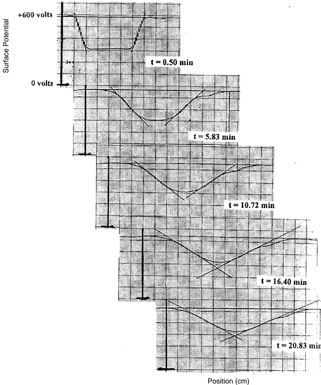
**Figure 2.** The electrostatic image structure of a positive-charging photoreceptor ( $22\ \mu\text{m}$ ) with a  $4\text{-}\mu\text{m}$  sol-gel overcoat<sup>6</sup> at 0.5, 5.83, 10.72, 16.40, and 20.83 min after exposure through a 0.25-cm slit. The position axis units are 0.051 cm/major division.
