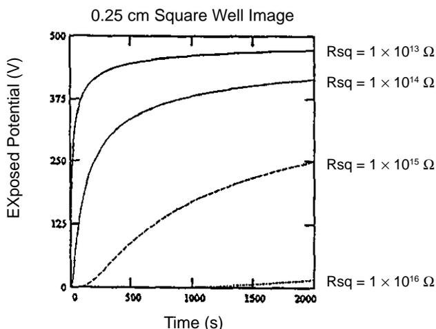
**Figure 8.** The surface potential at the exposed minimum of a 0.25-cm square-well image as a function of time after exposure for varied surface resistances calculated from Eq. 4.
