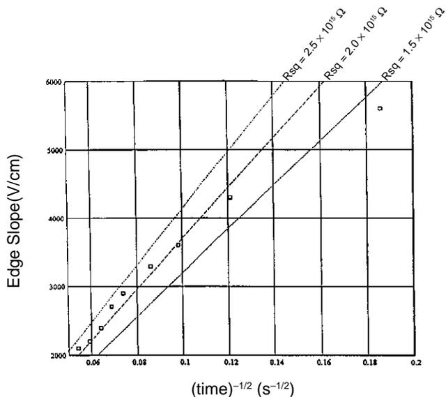
**Figure 7.** The image edge slopes (symbols) for a sol-gel-overcoated photoreceptor as a function of time (s) after exposure. The lines are calculated from Eq. 3, using the surface resistance values indicated. The best “eyeball fit” is with a surface resistance of  $3.0 \times 10^{15} \Omega$ .
