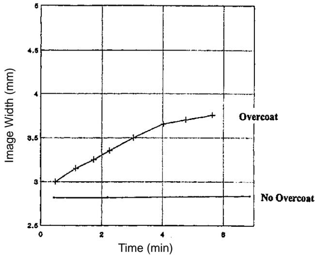
**Figure 3.** The square well image width as a function of time delay after exposure through a 0.25-cm slit for a nonovercoated and a sol-gel-overcoated<sup>6</sup> positive charging photoreceptor. The image width is defined as the distance, at the surface potential maximum, between the lines drawn tangent to the image edges.
