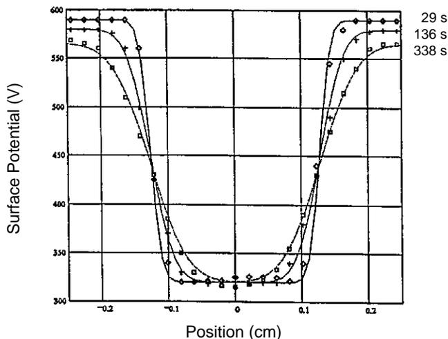
**Figure 6.** Experimental data (symbols) and image shapes calculated with Eq. 2 (curves) for a sol-gel-overcoated photoreceptor at 29, 136, and 338 s after exposure. The best “eyeball fit” to these data is with a surface resistance of  $3.0 \times 10^{15} \Omega$ .
