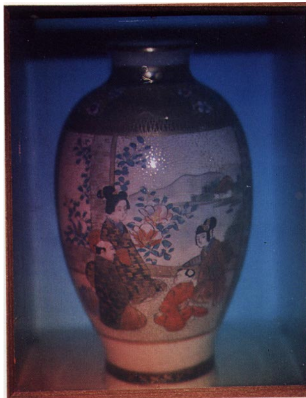
Figure 8. A 10 \times 12 -cm color hologram of a polychrome vase. The hologram was recorded with 477-, 532-, and 633-nm (blue, green, and red) laser wavelengths.
