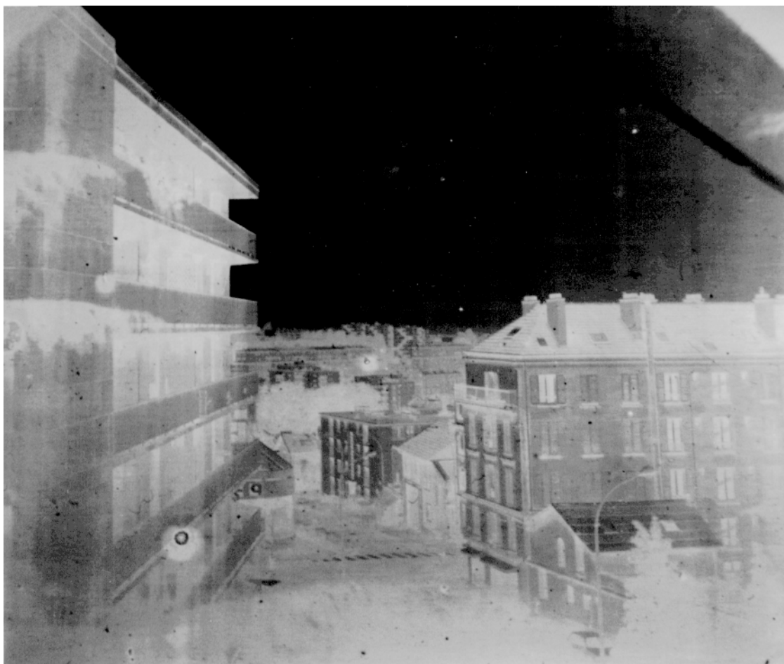
Photograph 4. The negative bitumen image of a heliograph made in a camera obscura in June 1990, under the same conditions as Niépce's. The line on the top right is the track of the sun, which rose during the morning. (© J. L. Marignier)
