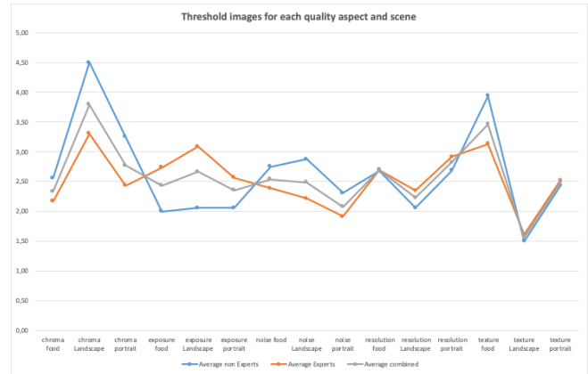
Figure 16: Selected last acceptable image for photographic applications sorted by expert and non-expert evaluation.
