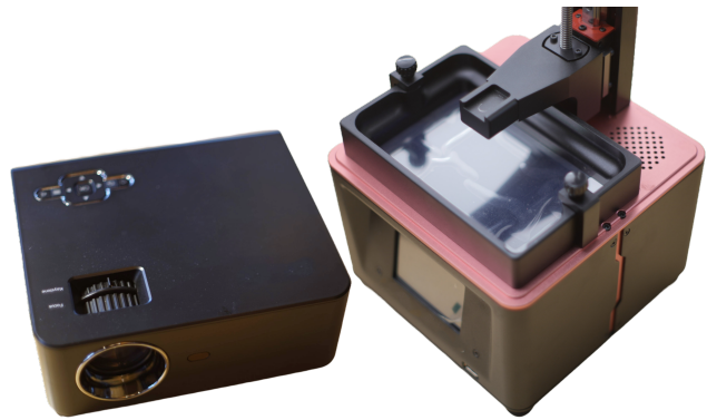
Figure 1. Transmissive LCDs are used in projectors and 3D printers
