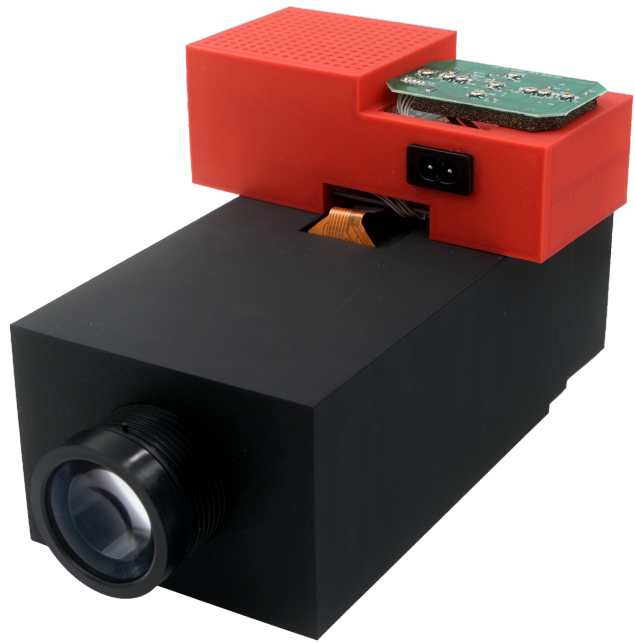
Figure 4. Kentucky LCD One Sensel (KLOS) camera
