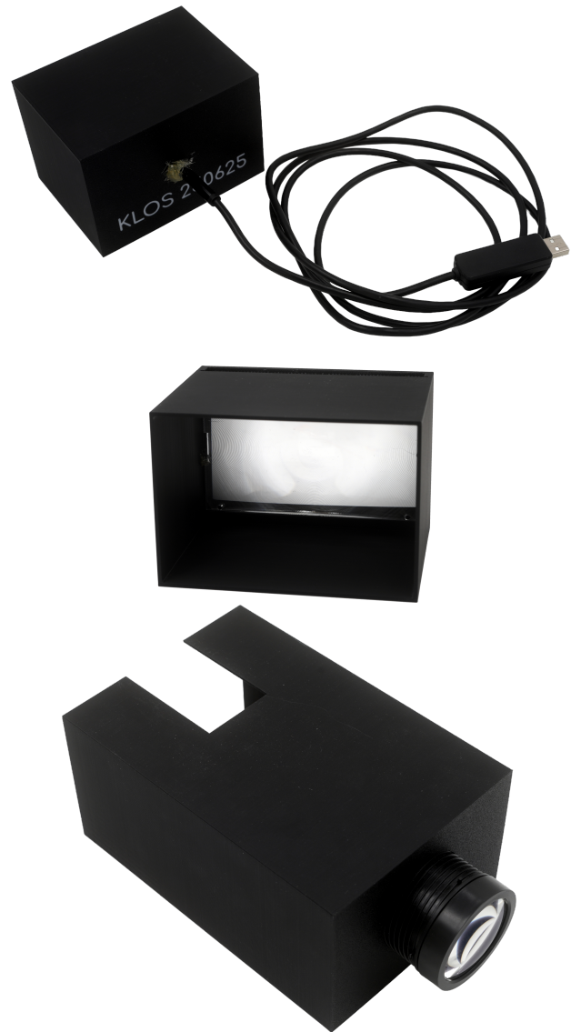
Figure 6. KLOS camera main modules
