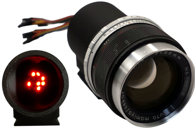
Figure 7. M42 CILKY: left: without lens, middle: with 55mm f/1.4 lens but no controller, right: projecting
