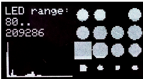
Figure 8. Ciro-flex CILKY's 128x64 pixel 0.96" OLED display
