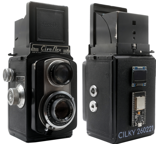
Figure 5. Ciro-flex CILKY captures IMEV TDCI data using a LED array
