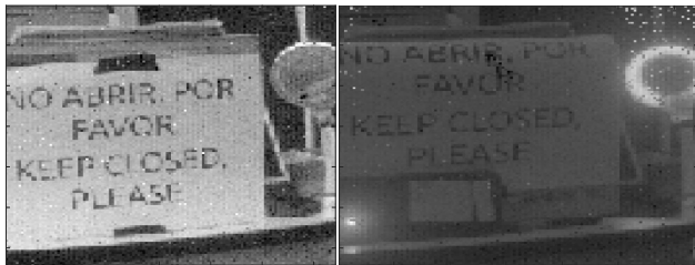
Figure 6. PVTTS High Intra-Dynamic Range, as pixels work independently.
