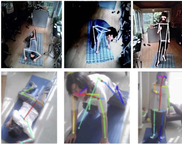
Figure 4. Extreme pose tracking of crawling, kneeling, and standing with LiDAR (up row) and webcam (bottom row)
