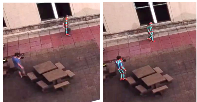
Figure 6. Gesture tracking results before the drone data fusion (left) and after the drone data fusion (right)
