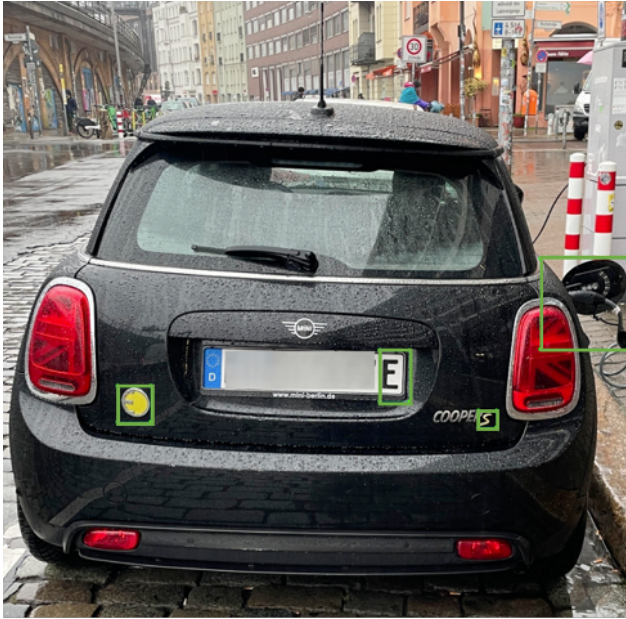
Figure 2. Example detection results showing EV-specific visual identifiers detected from rear-view vehicle images under urban conditions
